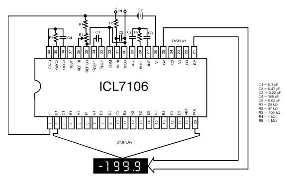
Figure 1. ICL7106 test circuit and typical application with LCD display components selected for 200mV full scale.
