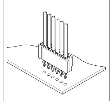
Measuring 2.0mm in pitch, 6.0mm in mounting height, and 3.25mm in thickness, this board-in connector meets the needs for high-density mounting on printed circuit boards efficiently and economically. The connector is ideal for VCRs, car stereo systems, audio products and many other consumer oriented electronic products.
