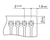
Note: 1. The above figure is the figure viewed from soldering side.
