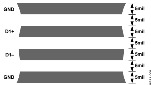
Figure 18. Arrangements of Signal Tracks
