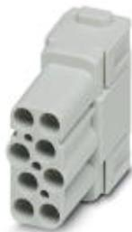
Contact insert module, number of positions: 8, power contacts: 8, control contacts: 0, Socket, Crimp connection, 400 V, 16 A, 0.5 mm<sup>2</sup> ... 4 mm<sup>2</sup>, application: Power
