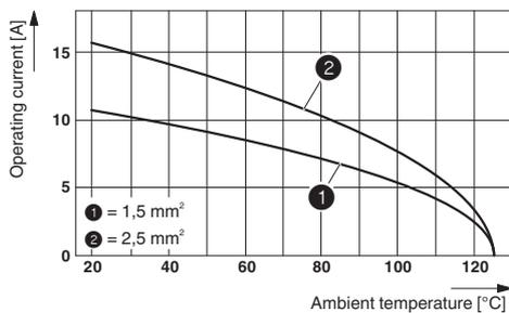
Derating diagram (6 modules in HC-B 24 housing)
