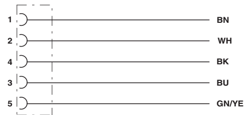
Contact assignment of the M12 socket
