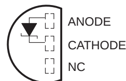
LP (TO-92/TO-226) PACKAGE (TOP VIEW)
