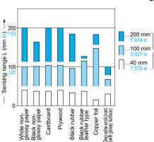
These bars indicate the sensing range with the respective objects when the distance adjuster is set to a sensing range of 200 mm 7.874 in, 100 mm 3.937 in and 40 mm 1.575 in long, respectively, with white non-glossy paper.
