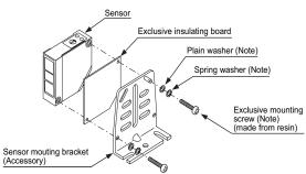
Note: Attached with the exclusive insulating board.
