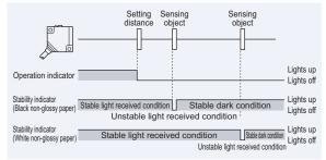
and not its intensity, the output corresponds to distance. The stability indicator displays the marginal degree of the incident light intensity. So take note that the distance by which the indicator lights on/off varies depending on the reflectance of the sensing object, as shown in the diagram below. Also, do not use the sensor when the stability indicator lights off
