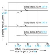
These curves show the characteristics with the maximum sensing range set to 200 mm 7.874 in, 100 mm 3.937 in and 40 mm 1.575 in, with white non-glossy paper (20 × 20 mm 0.787 × 0.787 in).
