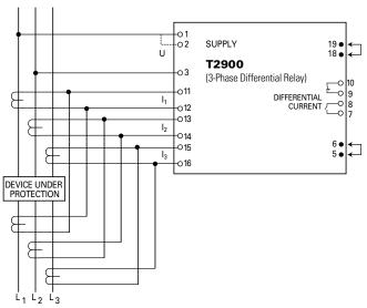
Bridge between terminals 5 and 6 results in latching relay. Bridge between terminals 18 and 19 reduces time delay to 0.1-1 sec.
