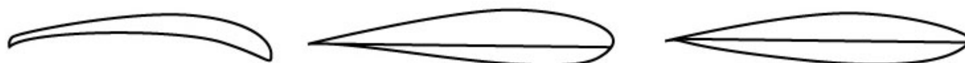
Custom-28 Profile, BP-28 NACA 44 Profile, BP-44 NACA 63 Profile, BP-63
