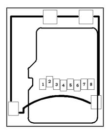
When removing the card, please make sure that you release it from the connector by pushing and NOT by pulling the card directly (this can damage both the connector and the microSD card).
