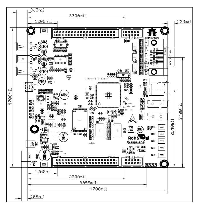
The three highest elements on the board in order from the tallest to the shortest are: capacitor C126 - 650mils, the three USB hosts -500mils, the VGA connector -475mils
