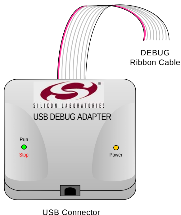
Figure 16. USB Debug Adapter
