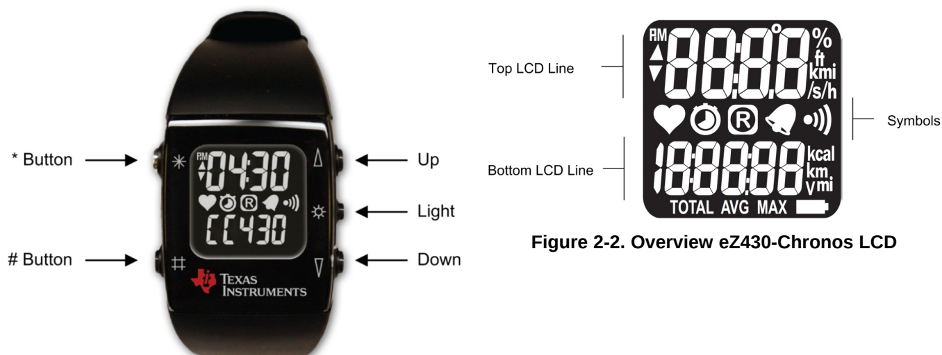
Figure 2-1. eZ430-Chronos Wrist Module Push Buttons
