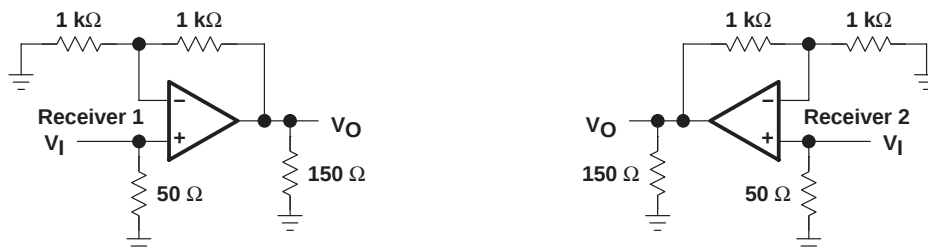
Figure 2. Receiver Input-to-Output Crosstalk Test Circuit
