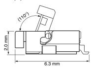
2. Front lock structure with tactile feedback
