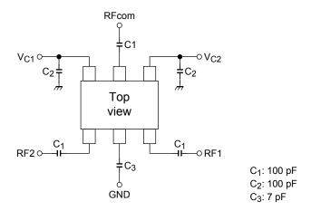
Please fix the value of each capacity for using frequency and circuit.
