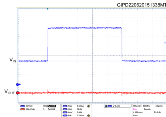
Figure 24: Line transient ( I_{OUT} = 0.8\text{ A} , V_{OUT} = 3\text{ V} )
