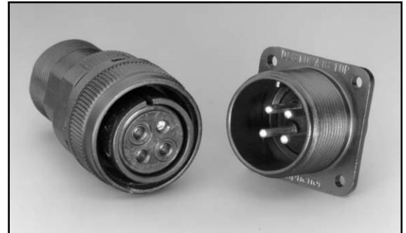
Amphenol® Pre-Earth FMLB Connectors Pre-Earth (ground) contact mates first and provides safety from voltage outputs - protects operators and sensitive circuits.
