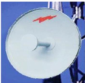
2.4 m | 8 ft Standard Parabolic Unshielded Antenna, single-polarized, unpressurized, 5.725–6.425 GHz, N Female, gray antenna, with flash, standard pack—one-piece reflector
