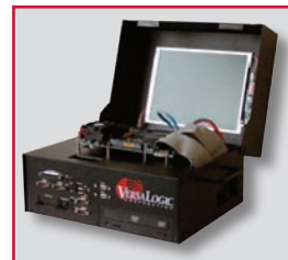
Optional cover (VL-ENCL-5LID) accommodates an SBC plus up to two PC/104 expansion modules. It provides protection for board-level components during storage or transport and a mounting location for flat panel displays.
