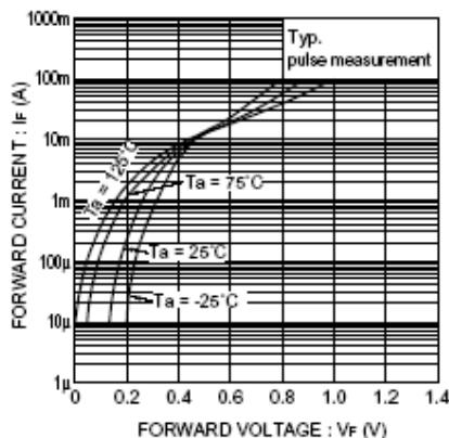
Fig. 1 Forward characteristics
