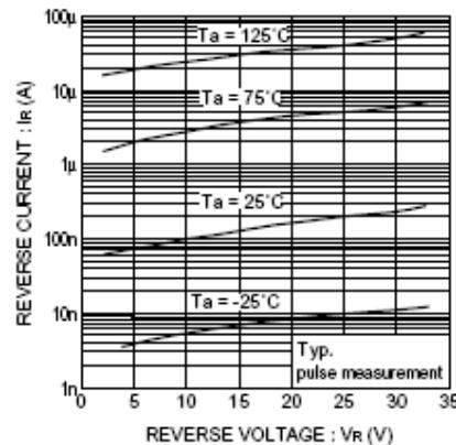
Fig. 2 Reverse characteristics
