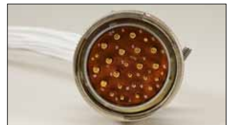
Connectors may contain several different size contacts.
