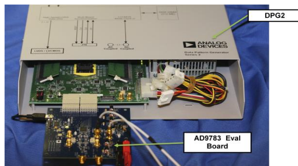
Figure 2- DPG2 and AD9783 Evaluation Board
