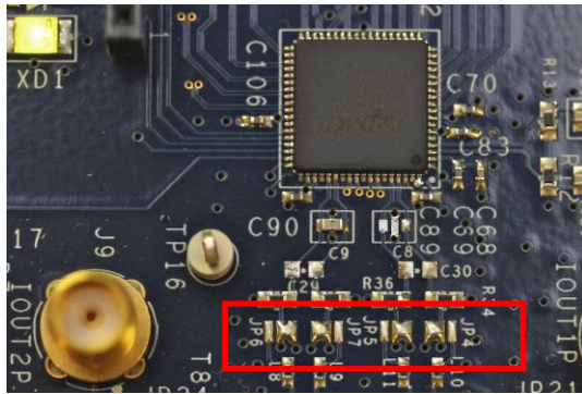
Figure 8 – a) DAC Output Configuration
