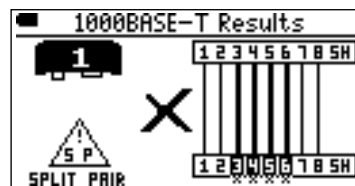
Typical split pair wiring fault
