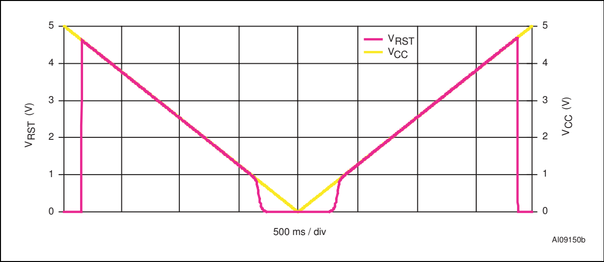
Figure 29. RST output voltage vs. supply voltage
