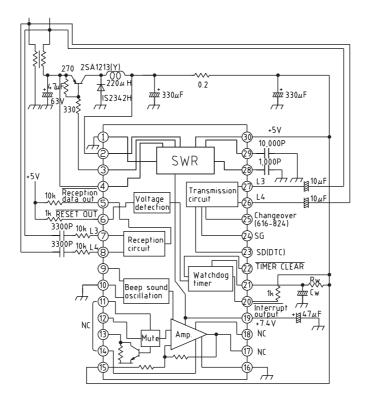
In order to prevent abnormal oscillation of the amplification circuit, a 5 V power supply must be connected to pin 15 to halt amplification functions.
