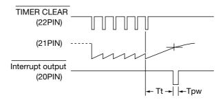
Note: Pulses to clear the timer must have a width of  $5\mu s$  or more.
