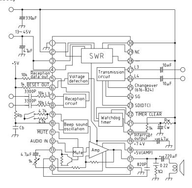
Even when a 5V external voltage can be supplied, an addition voltage of 13 to 45V must be applied to pins 3 and 4 in order to obtain an internal biased power supply of 7.4V.
