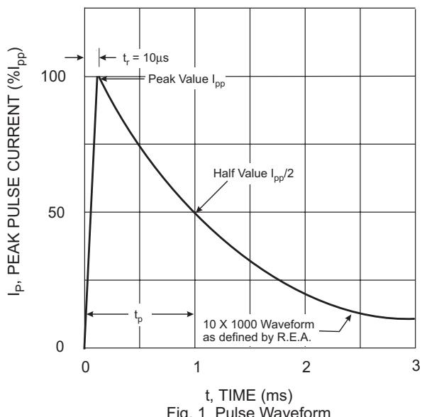
Fig. 1 Pulse Waveform
