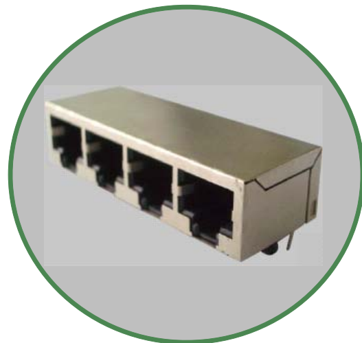
10/100 Mbps, Without LED, Latch-Down 8P, 8C, Shielded
