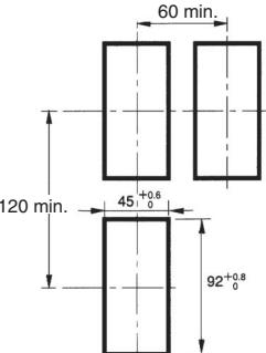
**Note:** 1. Recommended panel thickness is 1 to 8 mm.
