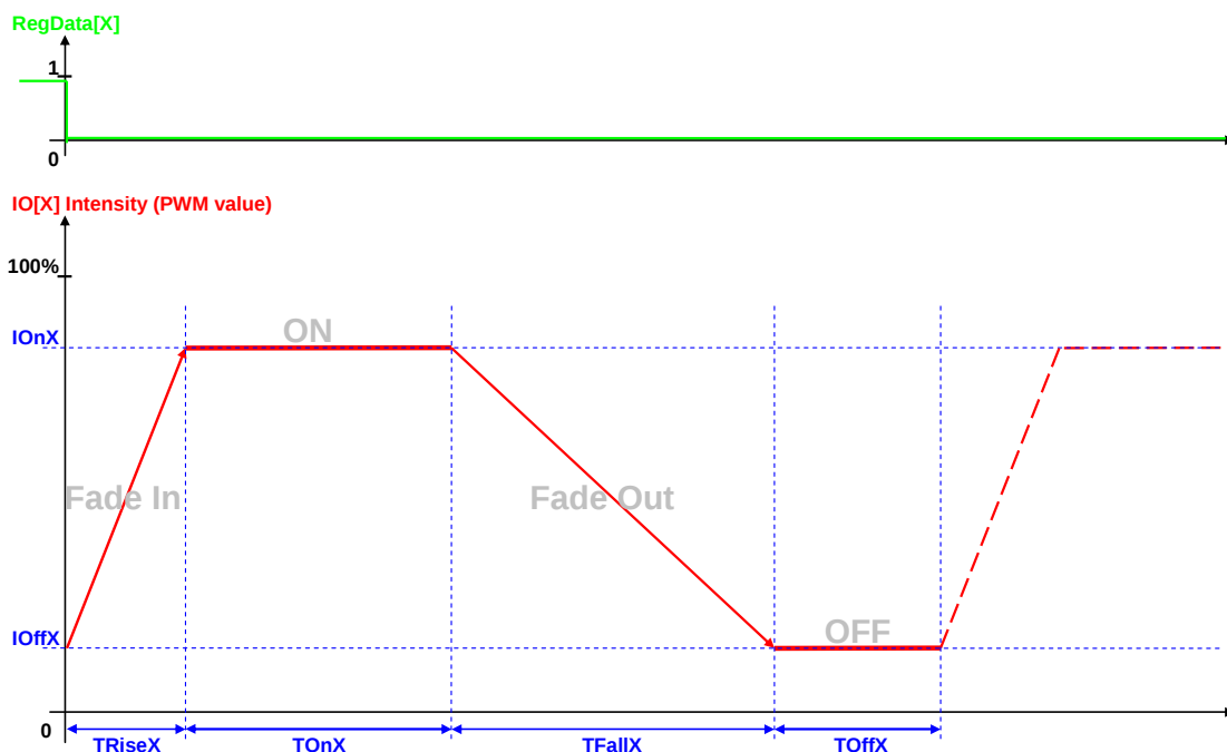
Figure 15 – LED Driver Overview
