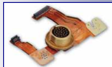
Flex Termination with MIL-C-26482 Special Connector
