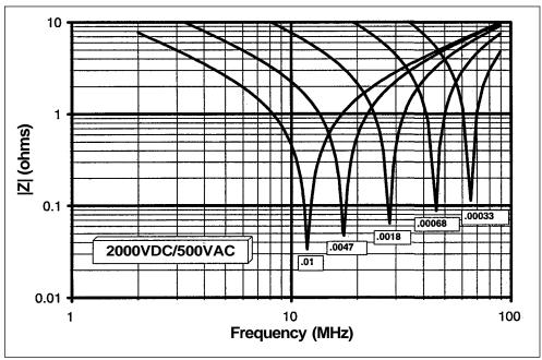
Please note: Capacitance values above are in  $\mu$ F The resonant frequency and impedance shown above apply to units with a 0.250 (6.4) lead length and are typical values only. Please contact us for additional data.
