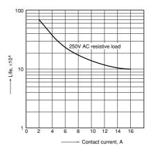
Notes: \*1. This value can change due to the switching frequency, environmental conditions, and desired reliability level, therefore it is recommended to check this with the actual load.
