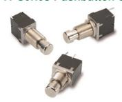
The single or double pole 641-Series represent the most compact offerings of our pushbutton switch line. Rugged metal construction, self cleaning contacts and stiff actuation force (3-3 1/2 lbs. typical) have made these switches ideal for most "foot pedal" type applications. These alternate action switches fit a standard .500" mounting hole, have termination options including solder lug, wire lead and PC, and are popular within the Music Industry and Audio-visual Markets.
