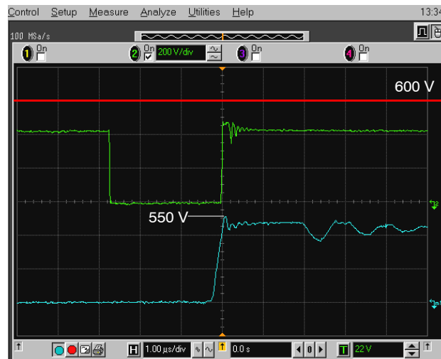
Figure 9. Maximum Output Power, V_{in} = 265 \text{ Vac} Note the good margin on the drain thanks to the low leakage term
