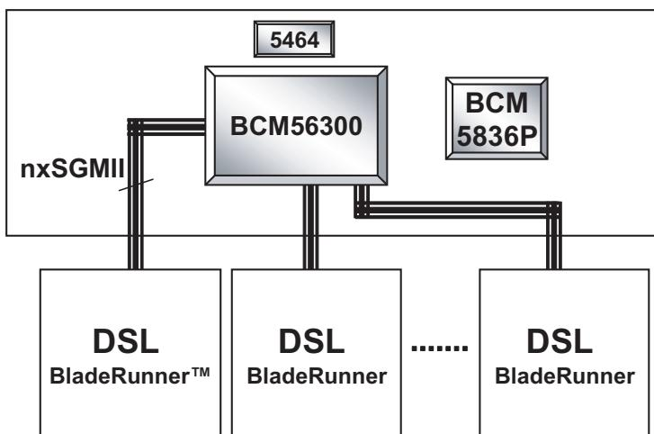
The BCM56300 is the fifth generation of the highly-integrated and cost-effective Broadcom StrataSwitch and StrataXGS product line in a single-chip solution with 24 GbE ports. The BCM56300 incorporates 24 GbE ports that can operate 10/100/1000 Mbps. The BCM56300 is a member of the Value GbE product line, with a corresponding pin compatible member in the Feature GbE product line—BCM56500.
