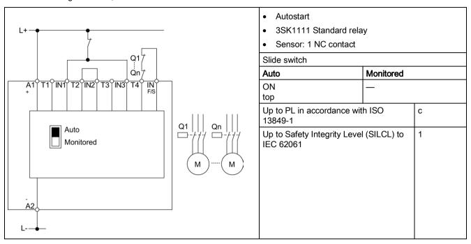
Table 7- 5 Typical circuit 5: 2-channel EMERGENCY STOP, with cross-circuit detection, with monitored start
