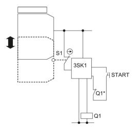
Figure 4-1 Single-channel sensor connection
