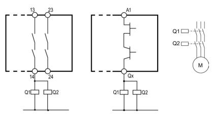
Figure 4-6 PL e/Cat. 4 in accordance with ISO 13849-1 or SILCL 3 in accordance with IEC 62061 With units that have solid-state outputs, this wiring is only possible from E02/V1.1.0.
