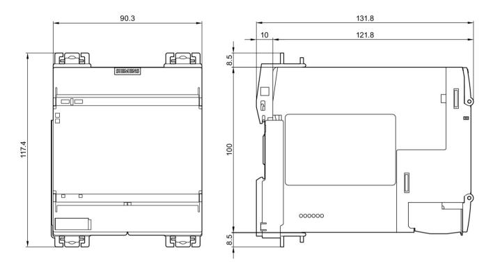
Figure 14-9 3SK1213 device on device connector
