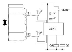
Figure 4-2 Two-channel sensor connection
