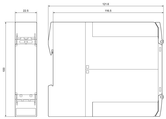
Figure 14-4 Enclosure 22.5 mm (long) for safety relays: 3SK1111-.....; 3SK1121-.....; 3SK1221-.....; 3SK1230-.....
