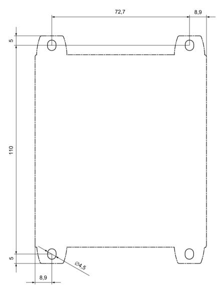
Figure 14-8 Drilling diagram, enclosure 90 mm
