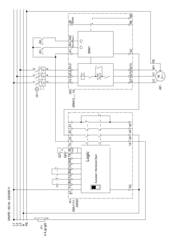
Figure 7-1 3SK1 safety relay with 3RM13 reversing starter
