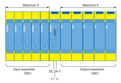
Example of a configuration with connection of 24 V DC on the basic unit and 3RM1 Failsafe motor starter
