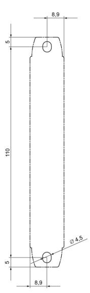
Figure 14-2 Drilling diagram, enclosure 17.5 mm
