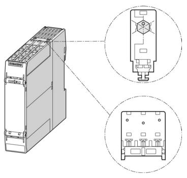
Figure 8-1 Module with coding pins
