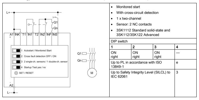
Table 7-9 Typical circuit 9: Two-channel, with cross-circuit detection, with autostart
