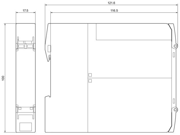
Figure 14-1 Enclosure 17.5 mm for safety relays: 3SK1120-.....; 3SK1220-.....
