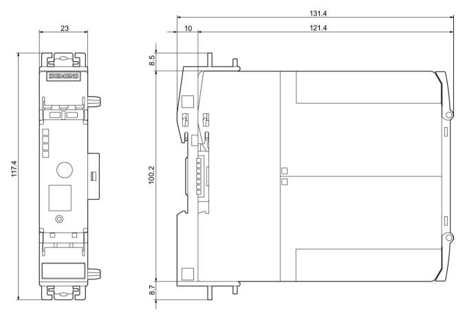
Figure 14-6 3SK1 device on device connector
