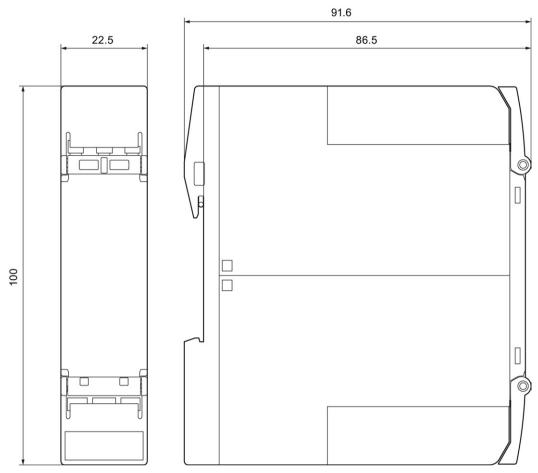
Figure 14-3 Enclosure 22.5 mm (short) for safety relays: 3SK1112-.....
