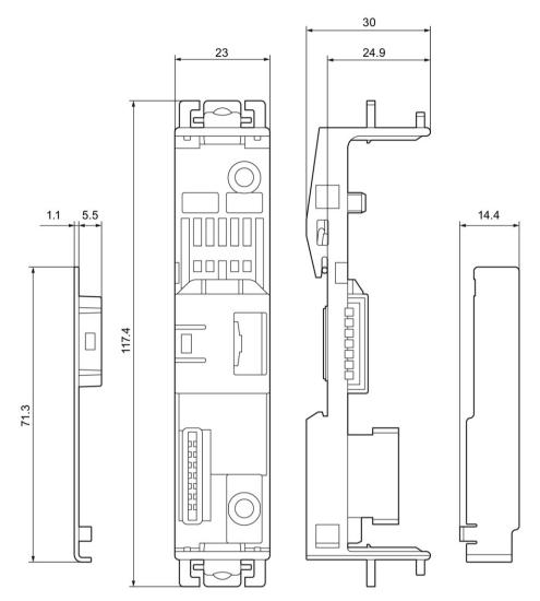
Figure 14-14 Device termination connector for 3RM1 motor starters, width: 22.5 mm
