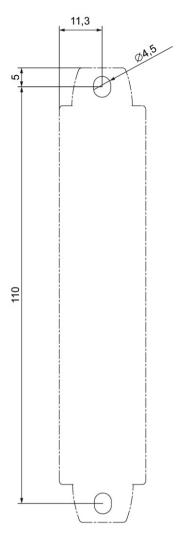
Figure 14-5 Drilling diagram, enclosure 22.5 mm
