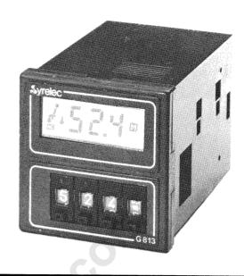
The 813 Timer is a multifunction control available in three different configurations. The basic control is the M,F or G mounting with one of four modes of operation slide switch selectable: Delay on Make, Single Shot, Delay on Break, and Repeat Cycle are standard. Normal and inverse relay operation is also slide switch selectable.
