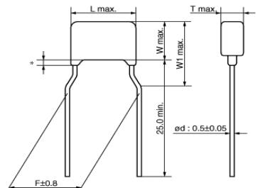
\* Coating extension does not exceed the end of the lead bend.
