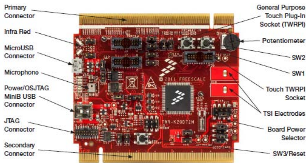
Figure 1. Front side of TWR-K20D72M module
