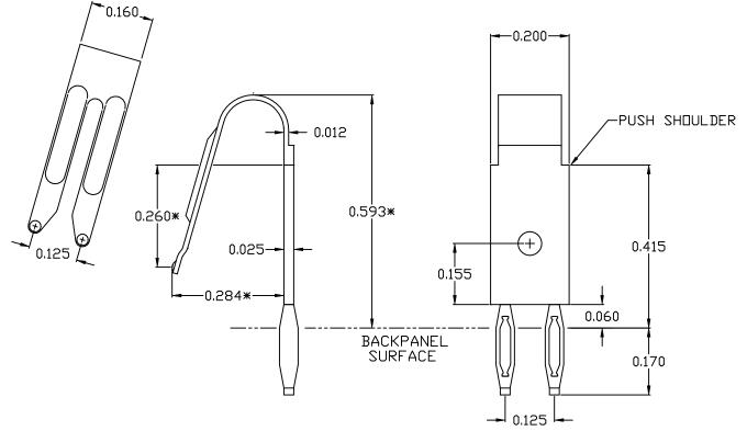
MATERIAL: C72500 PLATING: 100 MICROINCH MIN. GOLD OVER 100 MICROINCH MIN. NICKEL INSERTION FORCE INTO BACKPANEL: 50 LBS TYP (130 MAX) RETENTION FORCE IN BACKPANEL: 40 LBS TYP (20 MIN) FOR USE WITH 1C TYPE PINS AND 963 CONNECTORS INSERTION/REMOVAL HAND TOOL: 1023A
