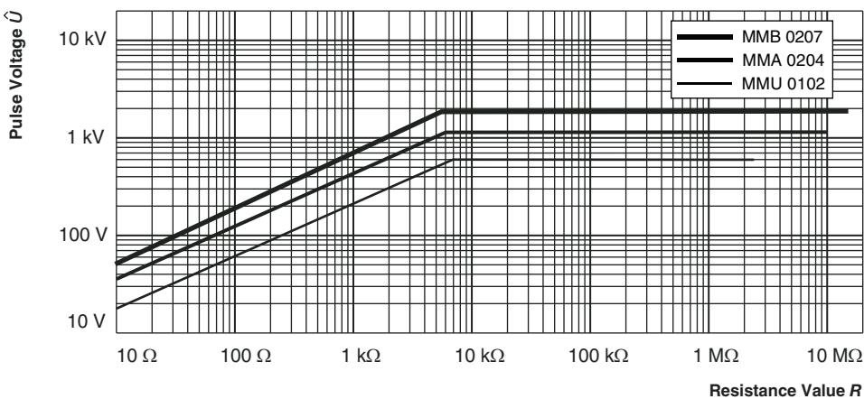
Pulse load rating in accordance with IEC 60115-1, 4.27; 10 μs / 700 μs;
