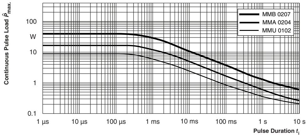
Maximum pulse load, continuous pulse; applicable if  $\bar{P} \leq P$  ( $\vartheta_{\text{amb}}$ ) and  $\hat{U} \leq \hat{U}_{\max.}$ ;
