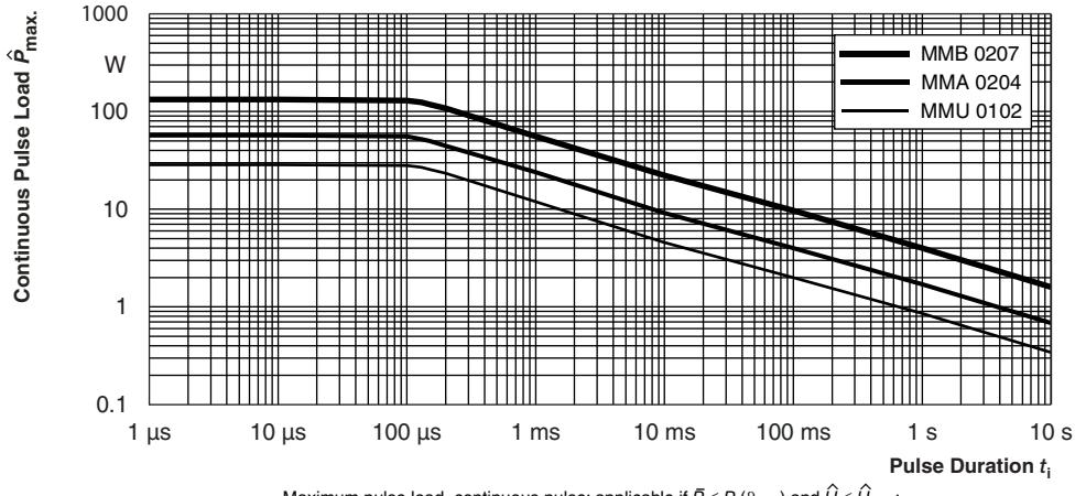
Maximum pulse load, continuous pulse; applicable if  $\bar{P} \leq P$  ( $\vartheta_{\text{amb}}$ ) and  $\hat{U} \leq \hat{U}_{\max.}$ ;
