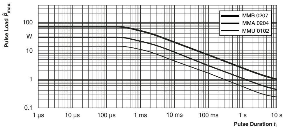
Maximum pulse load, single pulse; applicable if  $\bar{P} \rightarrow 0$  and  $n \leq 1000$  and  $\hat{U} \leq \hat{U}_{\text{max}}$ ;
