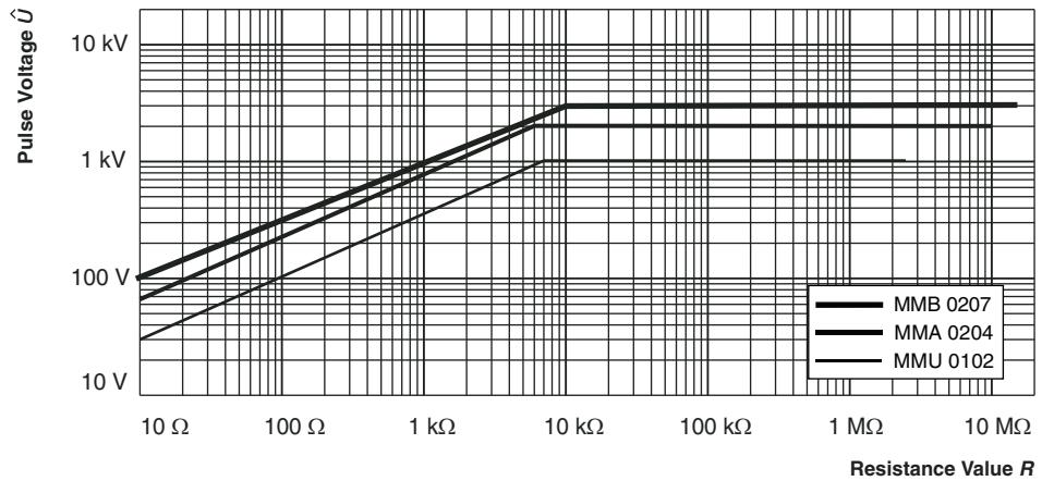
Pulse load rating in accordance with IEC 60 115-1, 4.27; 1.2 μs / 50 μs;
