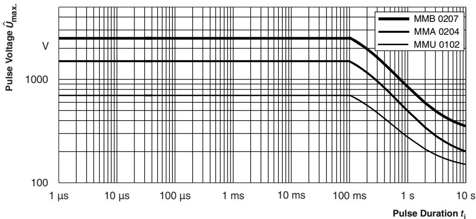
Maximum pulse voltage, single and continuous pulses; applicable if  $\hat{P} \leq \hat{P}_{\max}$ ;
