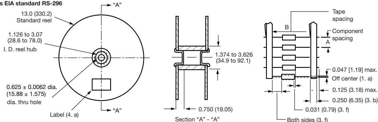
**STANDARD PACKAGING QUANTITY AND DIMENSIONS** in inches (millimeters)
