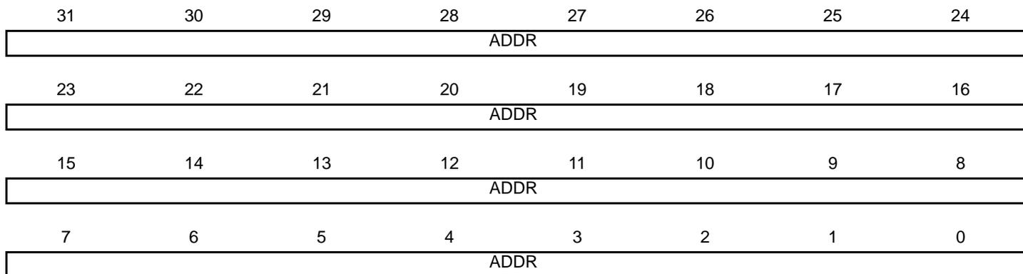
**ADDR: DMA Transfer Overlay 1 Address**
