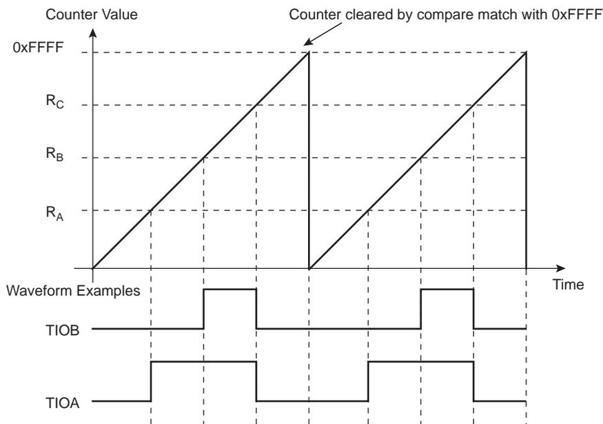
**Figure 46-8: WAVSEL = 00 with Trigger**
