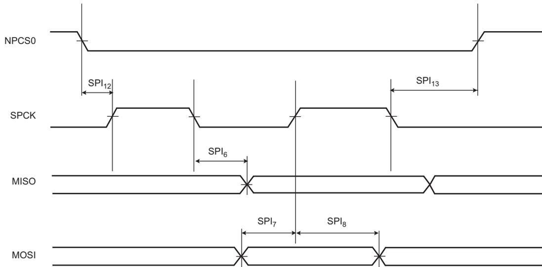
**Figure 56-28: USART SPI Slave Mode 0 or 3**
