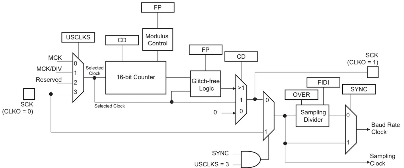
**Warning:** When the value of US\_BRGR.FP is greater than 0, the SCK (oversampling clock) generates nonconstant duty cycles. The SCK high duration is increased by “selected clock” period from time to time. The duty cycle depends on the value of USART\_BRGR.CD.
