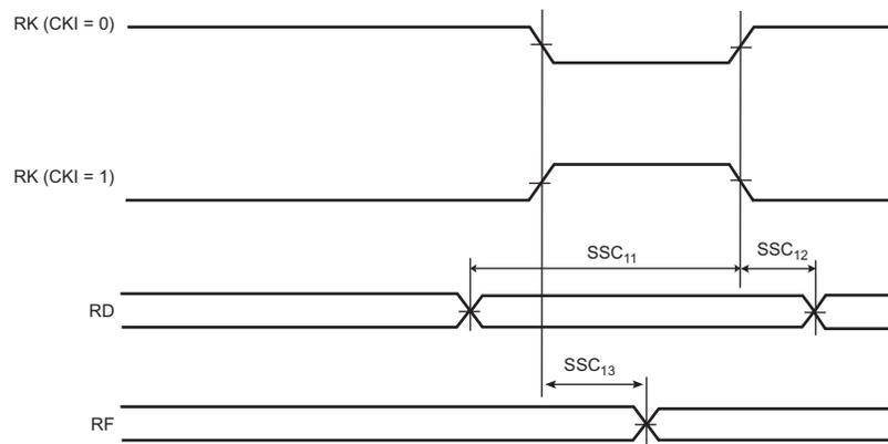
**Figure 56-20: SSC Receiver, RK in Output and RF in Input**
