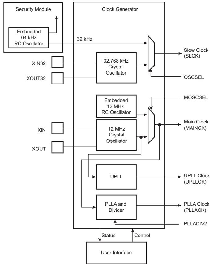
The embedded 64 kHz RC oscillator is always enabled when VDDBU is powered. The 12 MHz RC oscillator is always enabled when VDDCORE is powered.
