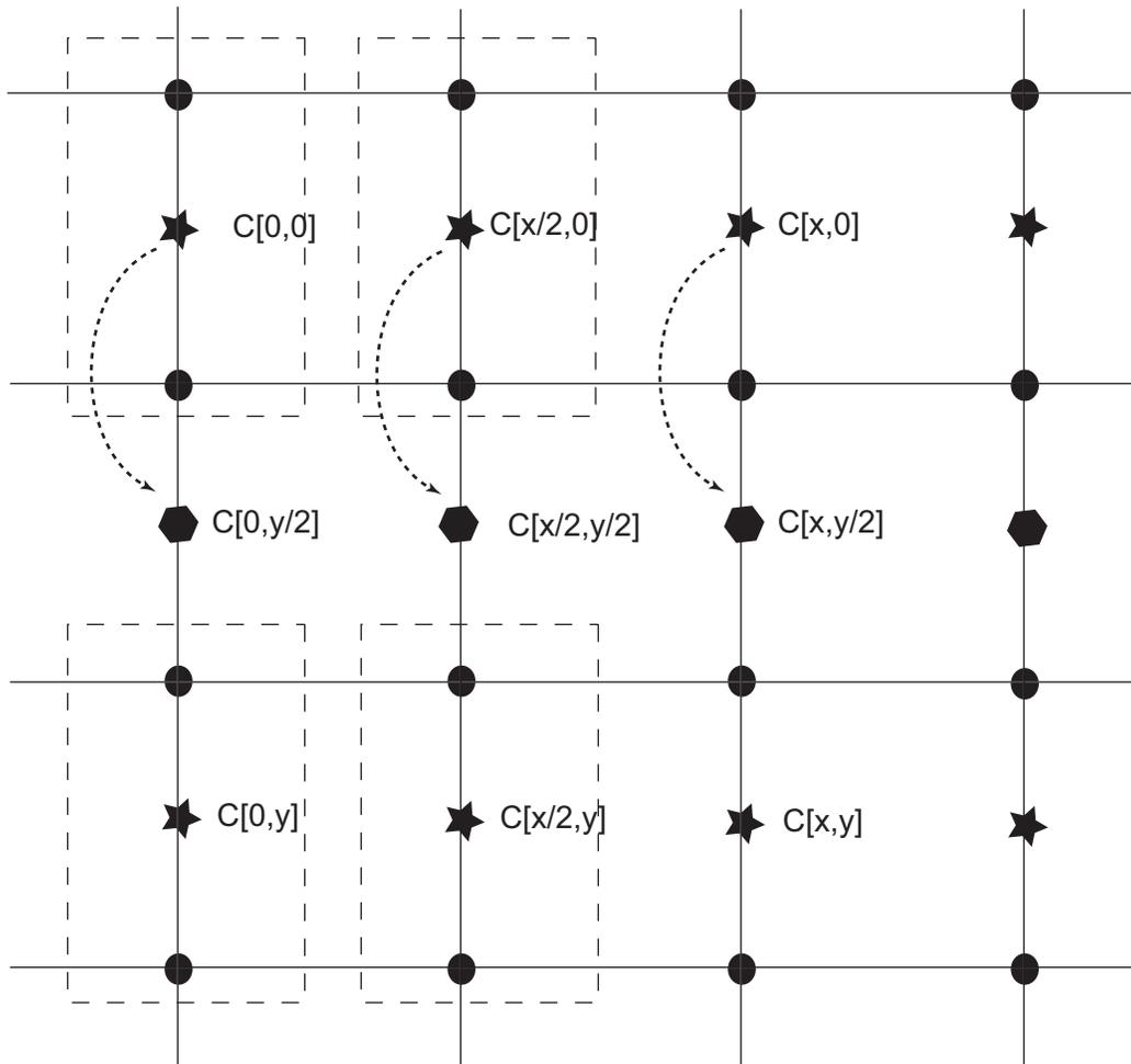
**Figure 32-4: 4:2:2 Semiplanar and Planar Upsampling Algorithm - 90 or 270 Degree R
