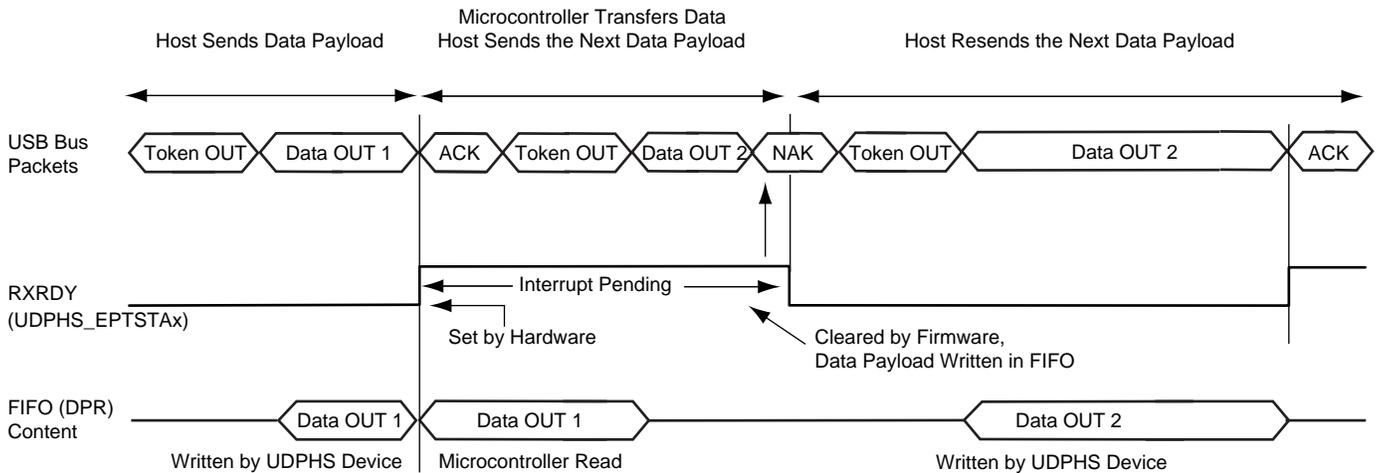
**Figure 35-15: Data OUT Transfer for an Endpoint with Two Banks**
