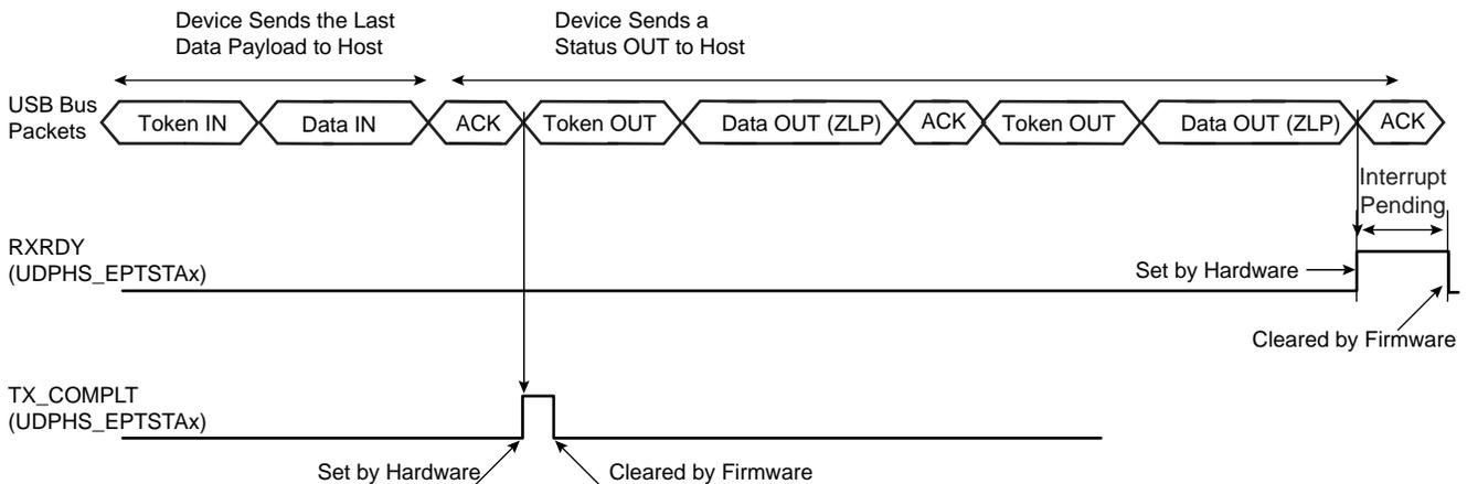
**Note:** A NAK handshake is always generated at the first status stage token.
