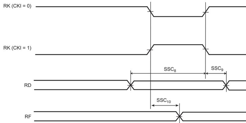
**Figure 56-19: SSC Receiver, RK and RF in Output**
