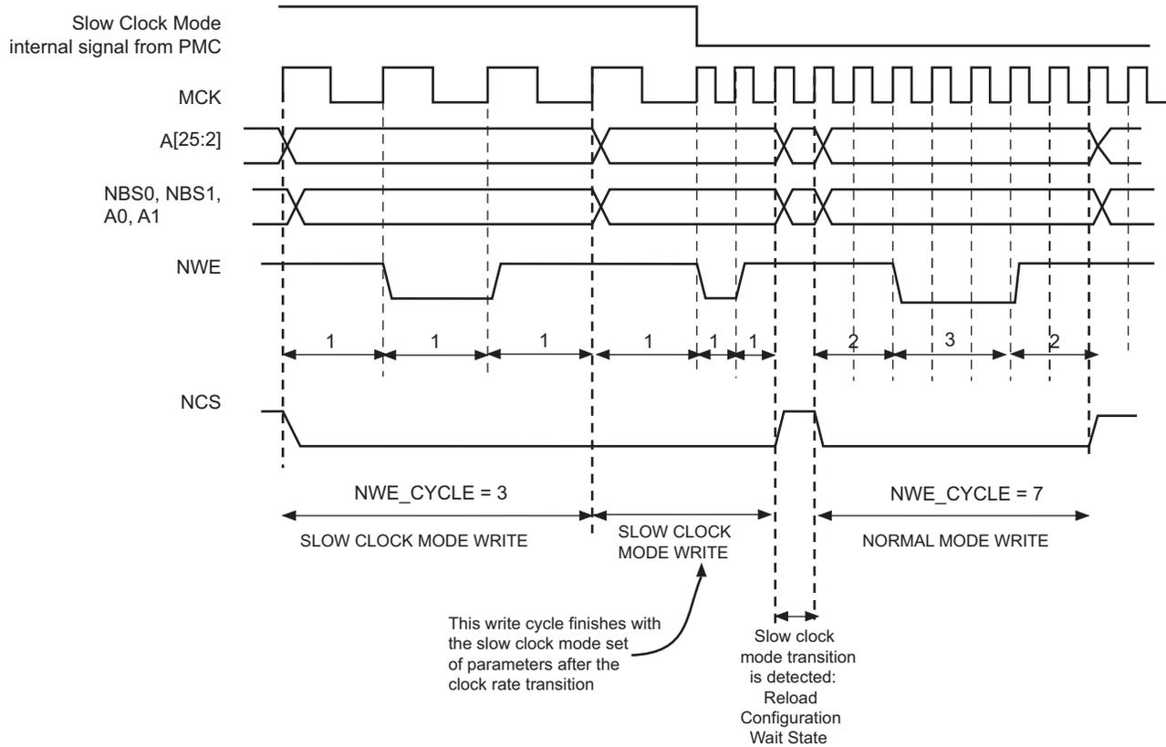
**Figure 30-30: Recommended Procedure to Switch from Slow Clock Mode to Normal Mode or from Normal Mode to Slow Clock Mode**
