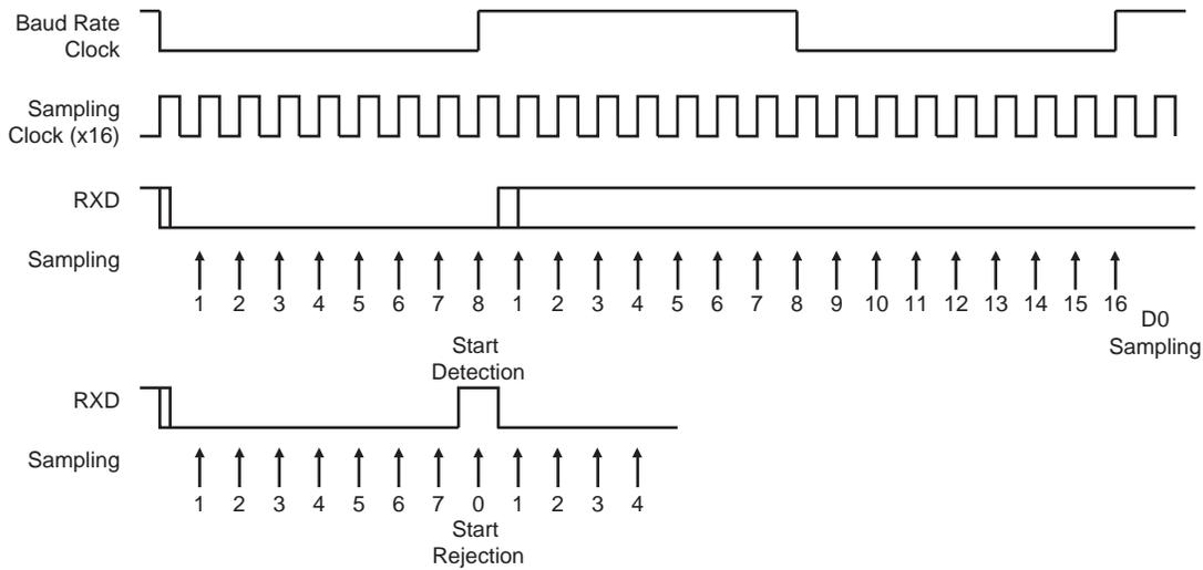
**Figure 44-12: Asynchronous Character Reception**
