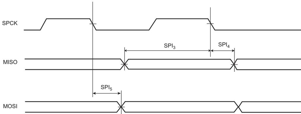
**Figure 56-8: SPI Slave Mode 0 and 3**
