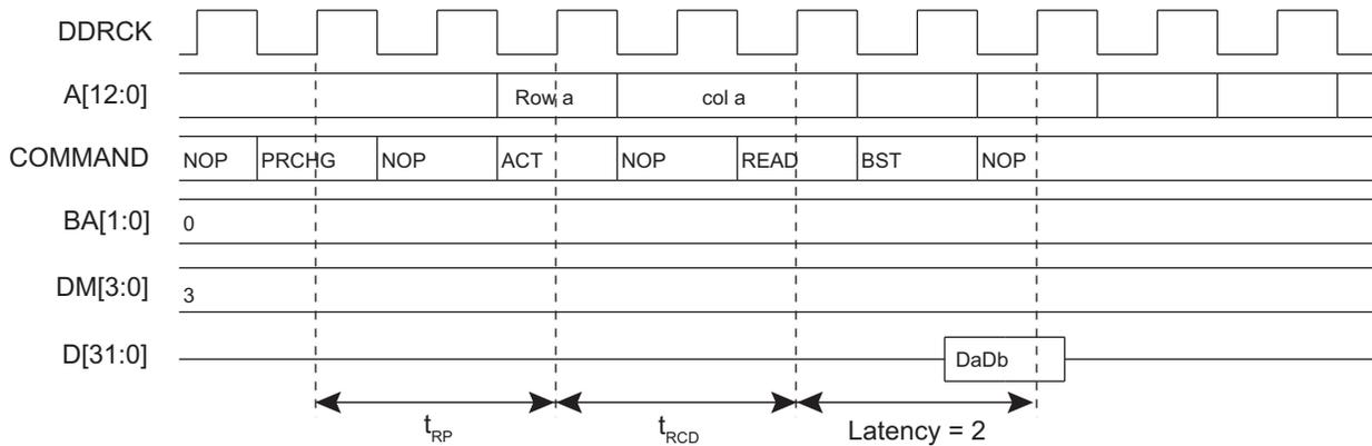
**Figure 29-10: Single Read Access, Row Closed, Latency = 3, DDR2-SDRAM Devices**
