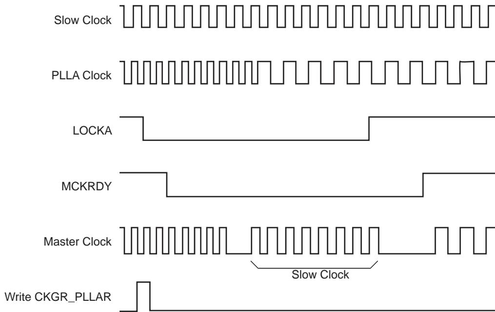
**Figure 27-10: Programmable Clock Output Programming**
