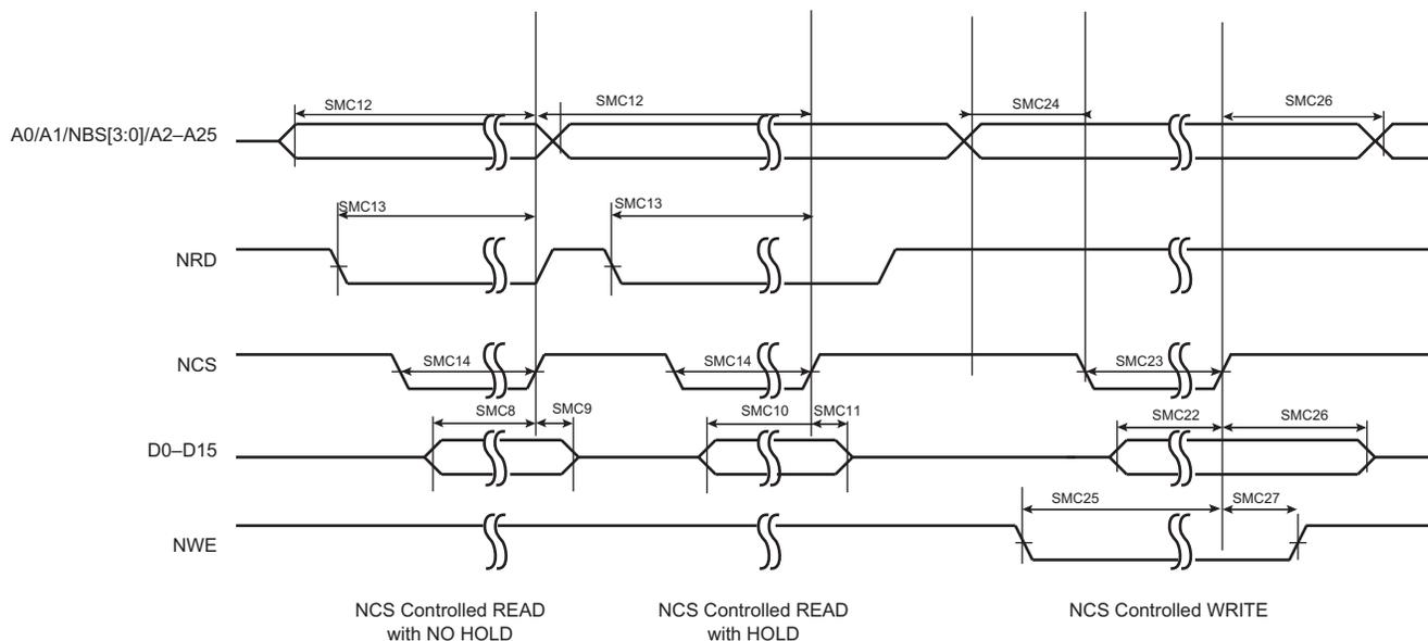
**Figure 56-5: SMC Timings - NRD Controlled Read and NWE Controlled Write**
