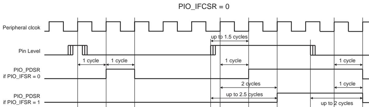
**Figure 28-5: Input Debouncing Filter Timing**
