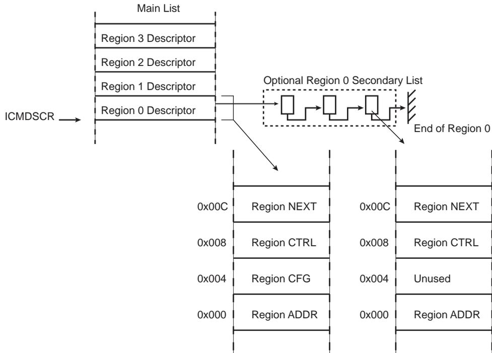
Figure 54-5 shows an example of the mandatory ICM settings to monitor three memory data blocks of the system memory (defined as two regions) with one region being not contiguous (two separate areas) and one contiguous memory area. For each said region, the SHA algorithm may be independently selected (different for each region). The wrap allows continuous monitoring.
