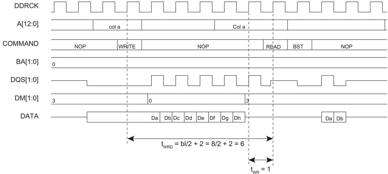
In case of a single write access, write operation should be interrupted by a read access but DM must be input 1 cycle prior to the read command to avoid writing invalid data. Refer to [Figure 29-7](#).
