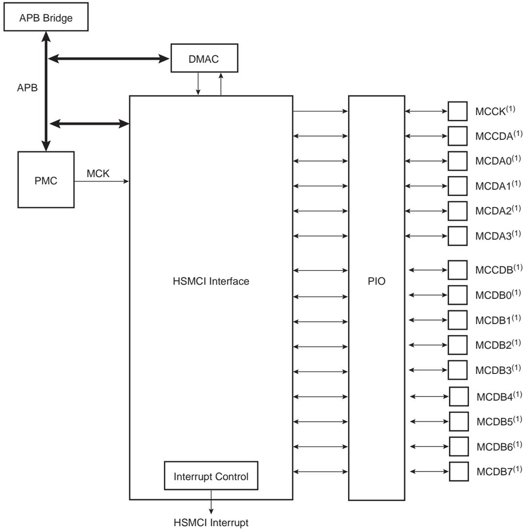
**Note 1:** When several HSMCI (x HSMCI) are embedded in a product, MCCK refers to HSMCIx\_CK, MCCDA to HSMCIx\_CDA, MCCDB to HSMCIx\_CDB, MCDAy to HSMCIx\_DaY, MCDBy to HSMCIx\_DBy.
