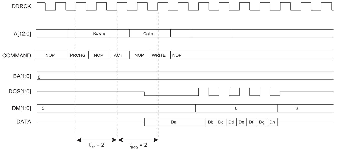
A write command can be followed by a read command. To avoid breaking the current write burst,  $t_{WTR}/t_{WRD}$  ( $bl/2 + 2 = 6$  cycles) should be met. Refer to [Figure 29-6](#).
