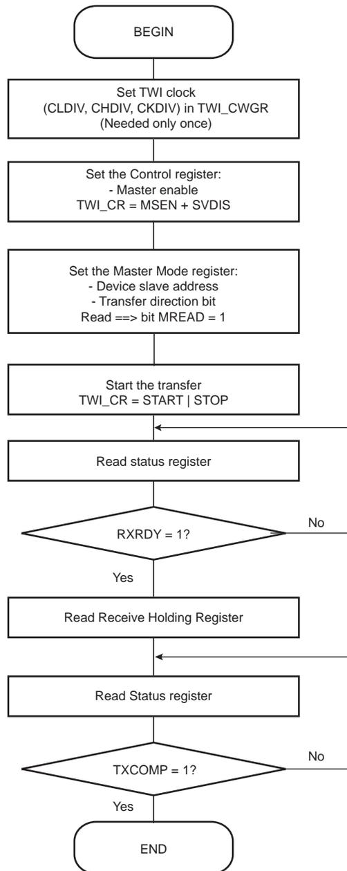
Figure 40-17: TWI Read Operation with Single Data Byte and Internal Address
