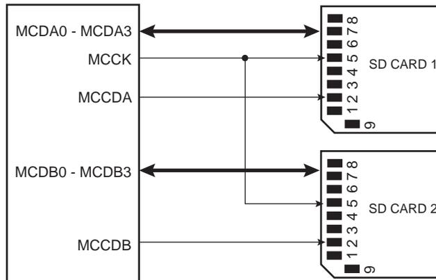
**Note:** When several HSMCI (x HSMCI) are embedded in a product, MCKK refers to HSMCIx\_CK, MCCDA to HSMCIx\_CDA, MCDAy to HSMCIx\_DAy, MCCDB to HSMCIx\_CDB, MCDBy to HSMCIx\_DBy.
