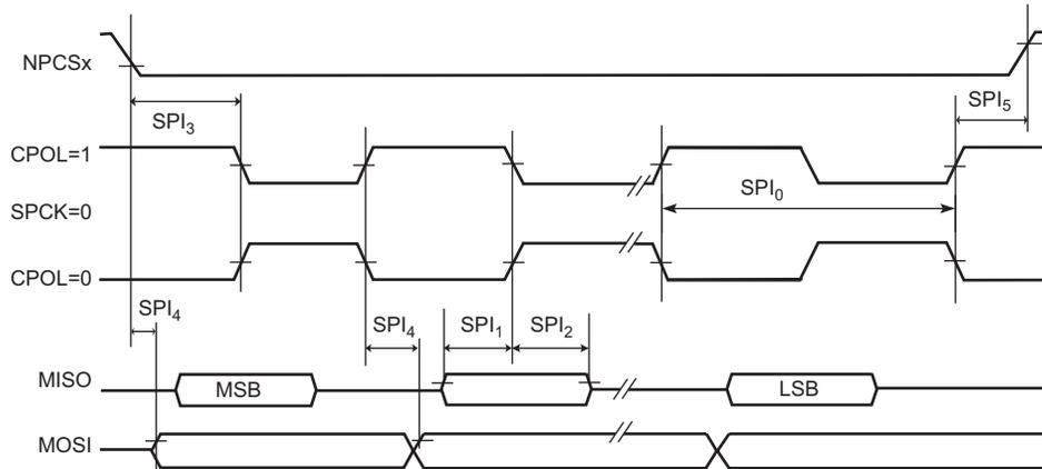
Figure 56-27: USART SPI Slave Mode 1 or 2
