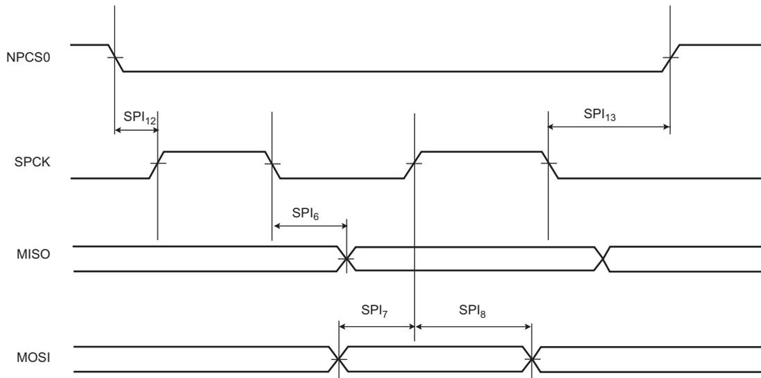
**Figure 56-9: SPI Slave Mode 1 and 2**
