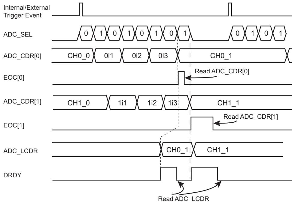
Note: ADC\_SEL: Command to the ADC analog cell
