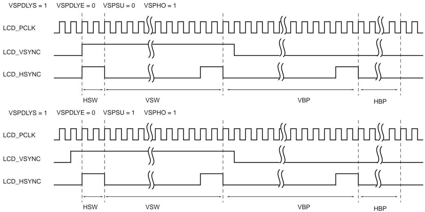
**Figure 32-18: DISP Signal Timing Diagram**
