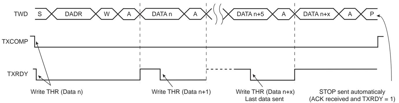
**Figure 40-6: Master Write with One Byte Internal Address and Multiple Data Bytes**
