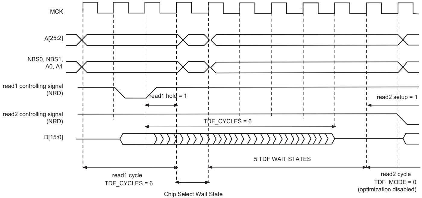
**Figure 30-21: TDF Mode = 0: TDF wait states between a read and a write access on different chip selects**
