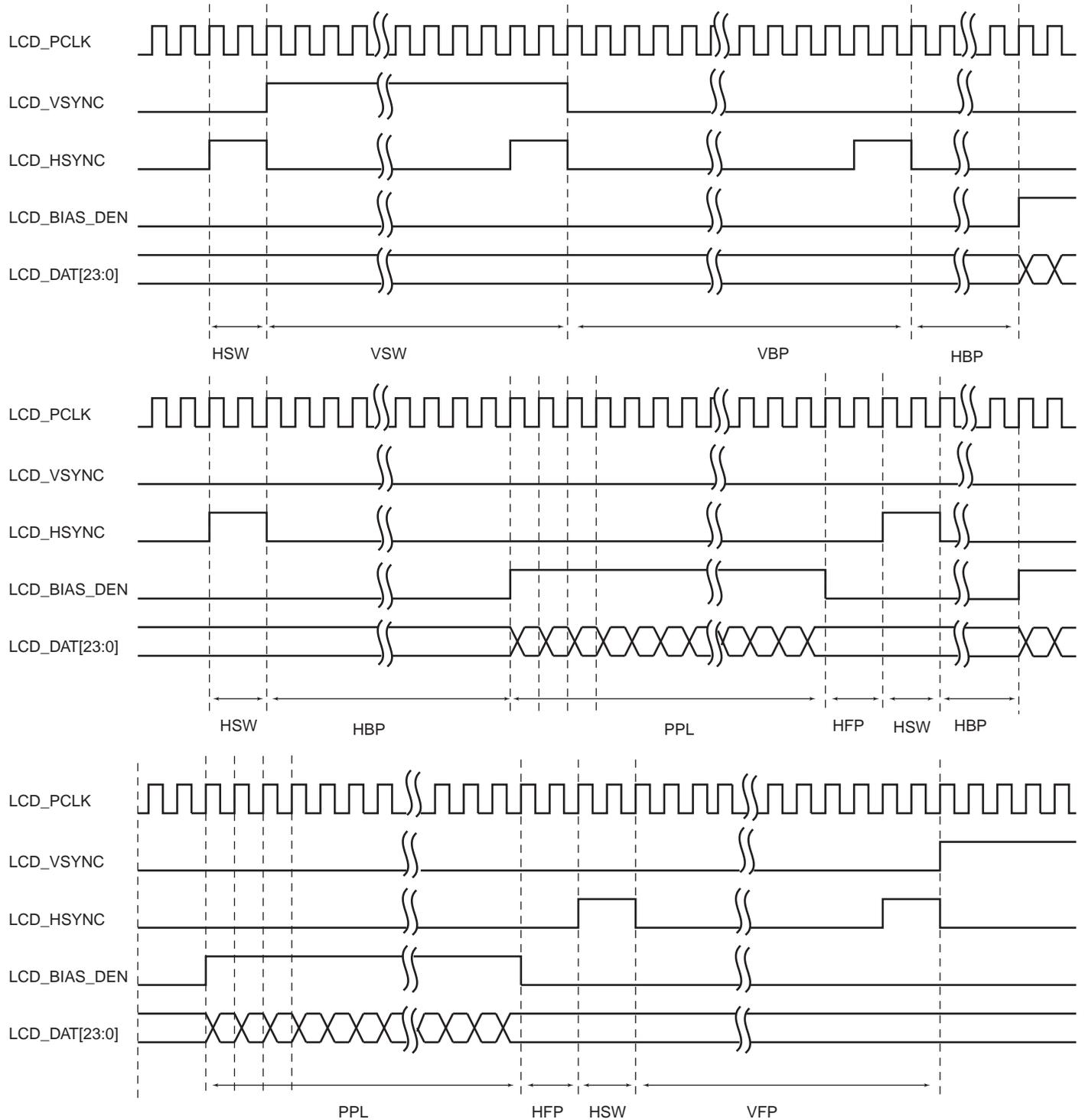
**Figure 32-16: Vertical Synchronization Timing (part 1)**
