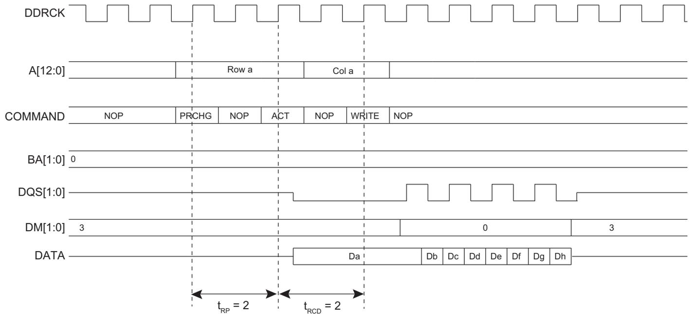
**Figure 29-5: Burst Write Access, Row Closed, DDR2-SDRAM Devices**
