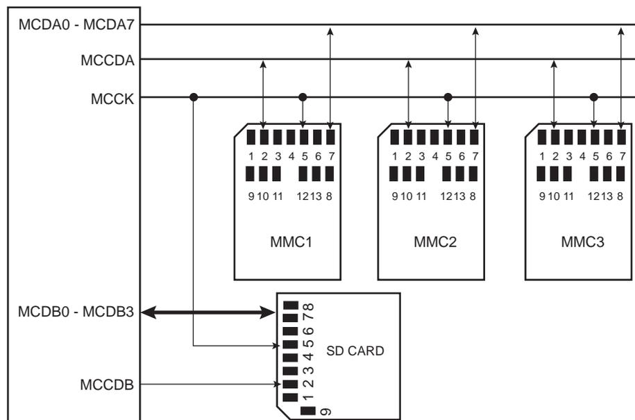
**Note:** When several HSMCI (x HSMCI) are embedded in a product, MCCK refers to HSMCIx\_CK, MCCDA to HSMCIx\_CDA, MCDAy to HSMCIx\_DaY, MCCDB to HSMCIx\_CDB, MCDBy to HSMCIx\_DBy.
