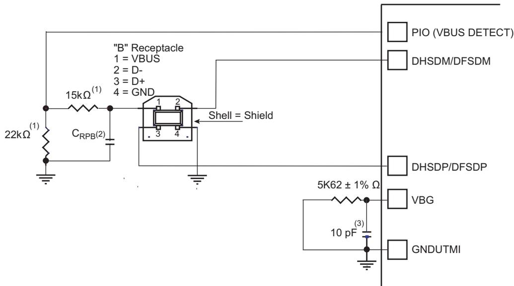
**Note 1:** The values shown on the 22 kΩ and 15 kΩ resistors are only valid with 3V3-supplied PIOs.
