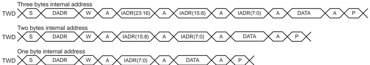
**Figure 40-11: Master Read with One, Two or Three Bytes Internal Address and One Data Byte**
