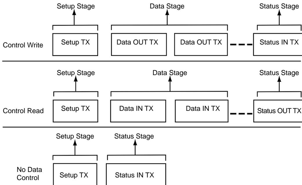
A status IN or OUT transaction is identical to a data IN or OUT transaction.
