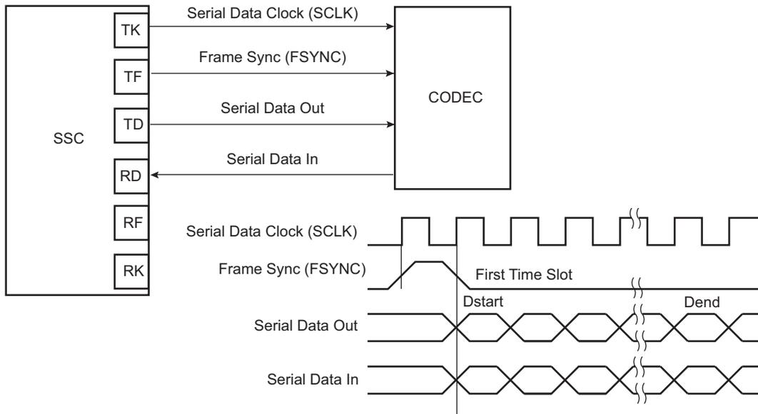
**Figure 41-5: Time Slot Application Block Diagram**
