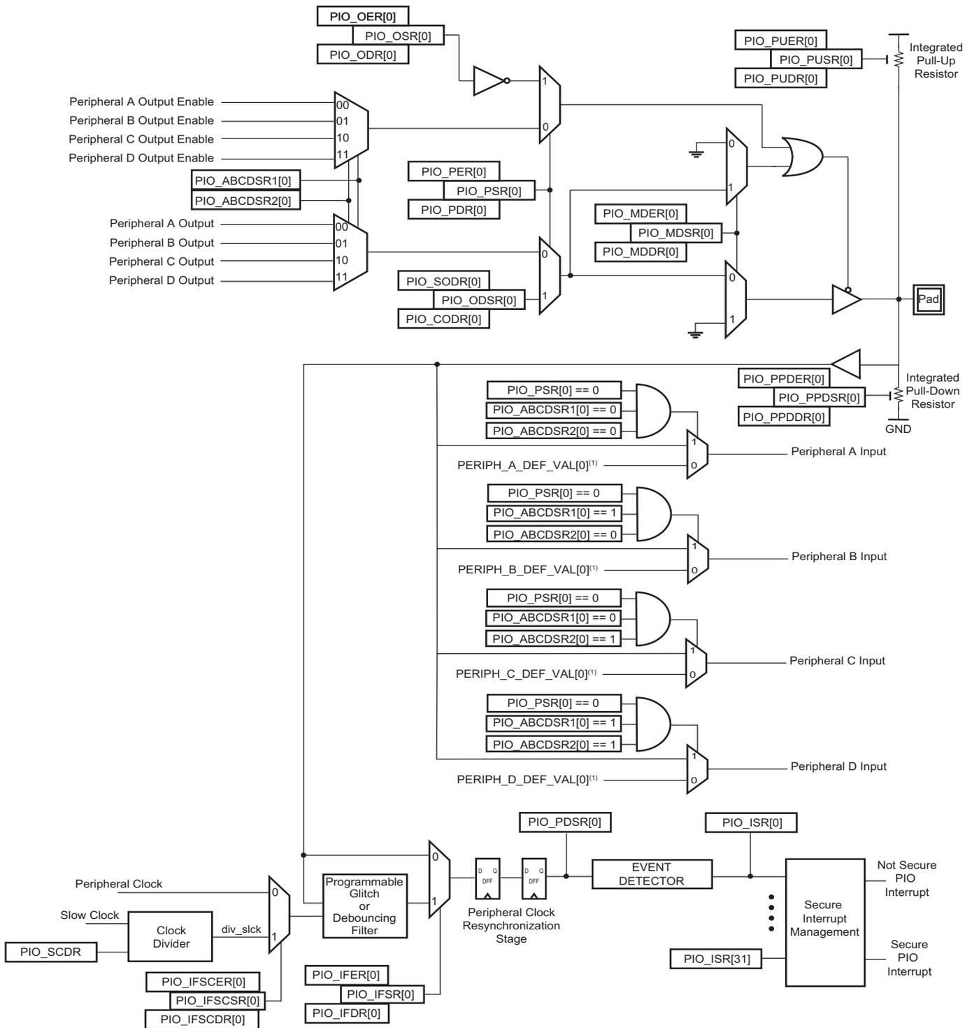
**Note 1:** PERIPH\_A\_DEF\_VAL = 0x00000000, PERIPH\_B\_DEF\_VAL = 0x00000000, PERIPH\_C\_DEF\_VAL = 0x00000000, PERIPH\_D\_DEF\_VAL = 0x00000000.
