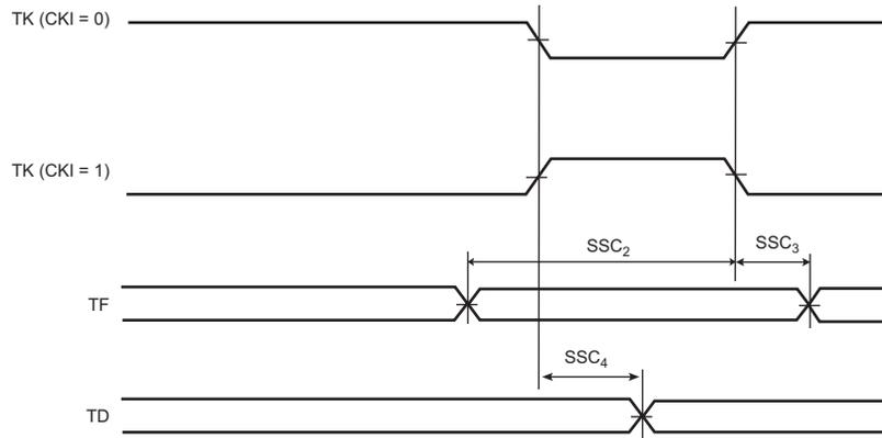
Figure 56-16: SSC Transmitter, TK and TF in Input
