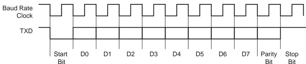
The characters are sent by writing in US\_THR. The transmitter reports two status bits in the Channel Status register (US\_CSR): TXRDY (Transmitter Ready), which indicates that US\_THR is empty, and TXEMPTY, which indicates that all the characters written in US\_THR have been processed. When the current character processing is completed, the last character written in US\_THR is transferred into the Shift register of the transmitter and US\_THR becomes empty, thus TXRDY rises.
