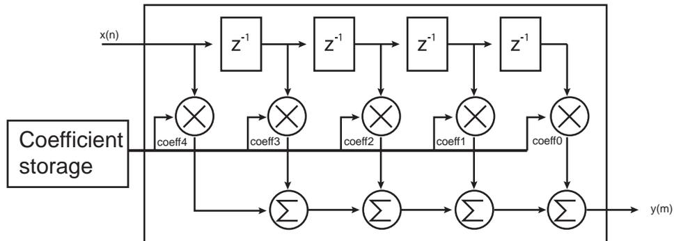
**Figure 32-8: Vertical Resampler Filter Architecture**
