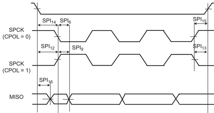
Table 56-37: SPI Timings with 3.3V Peripheral Supply
