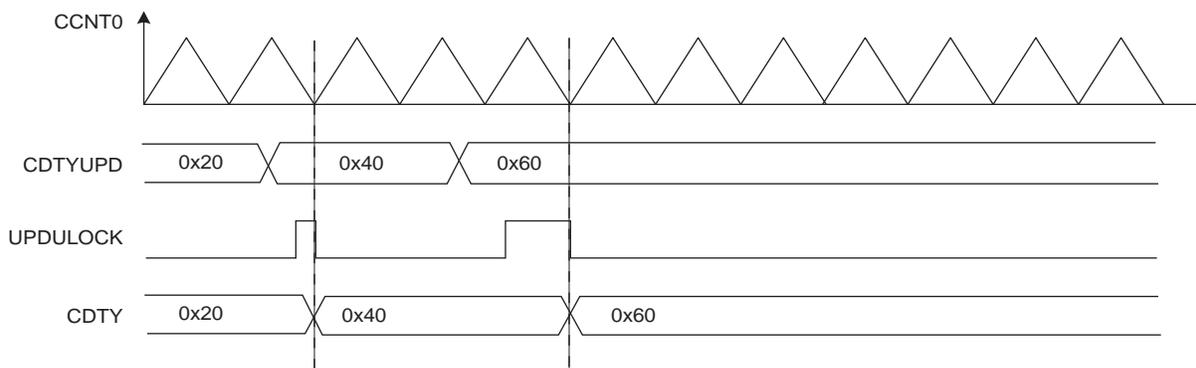
*Method 2: Manual write of duty-cycle values and automatic trigger of the update*
