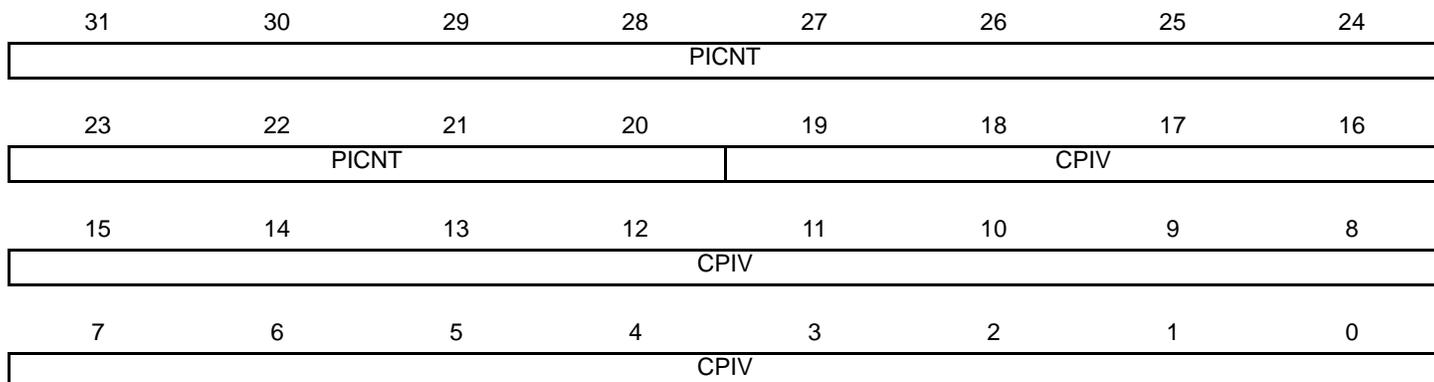
Reading this register clears PITS in PIT\_SR.
