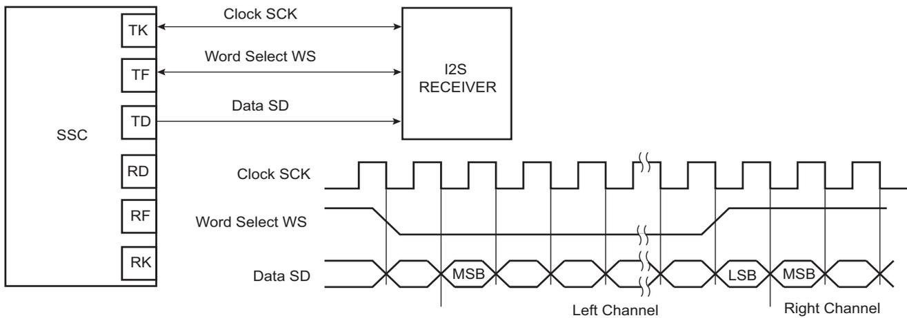
**Figure 41-4: Codec Application Block Diagram**
