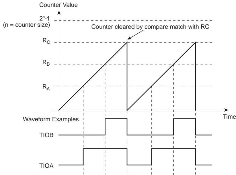
**Figure 46-10: WAVSEL = 10 with Trigger**
