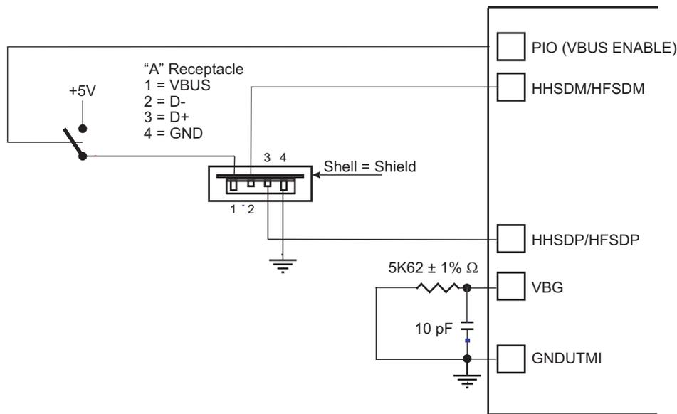
3: Typical USB High Speed Device connection:
