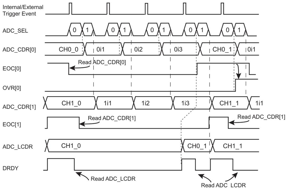
Notes: ADC\_SEL: Command to the ADC analog cell
