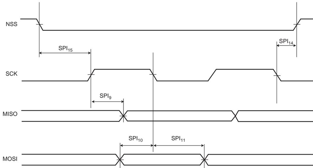
**Table 56-52: USART SPI Timings 3.3V Peripheral Supply**
