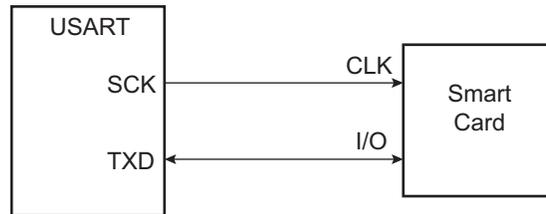
When operating in ISO7816, either in T = 0 or T = 1 modes, the character format is fixed. The configuration is 8 data bits, even parity and 1 or 2 stop bits, regardless of the values programmed in the Mode register fields CHRL, MODE9, PAR and CHMODE. US\_MR.MSBF can be used to transmit LSB or MSB first. US\_MR.PAR can be used to transmit in Normal or Inverse mode. Refer to [Section 44.7.3 “USART Mode Register”](#) and [“PAR: Parity Type”](#).
