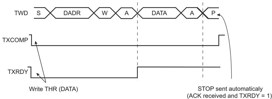
**Figure 40-5: Master Write with Multiple Data Bytes**
