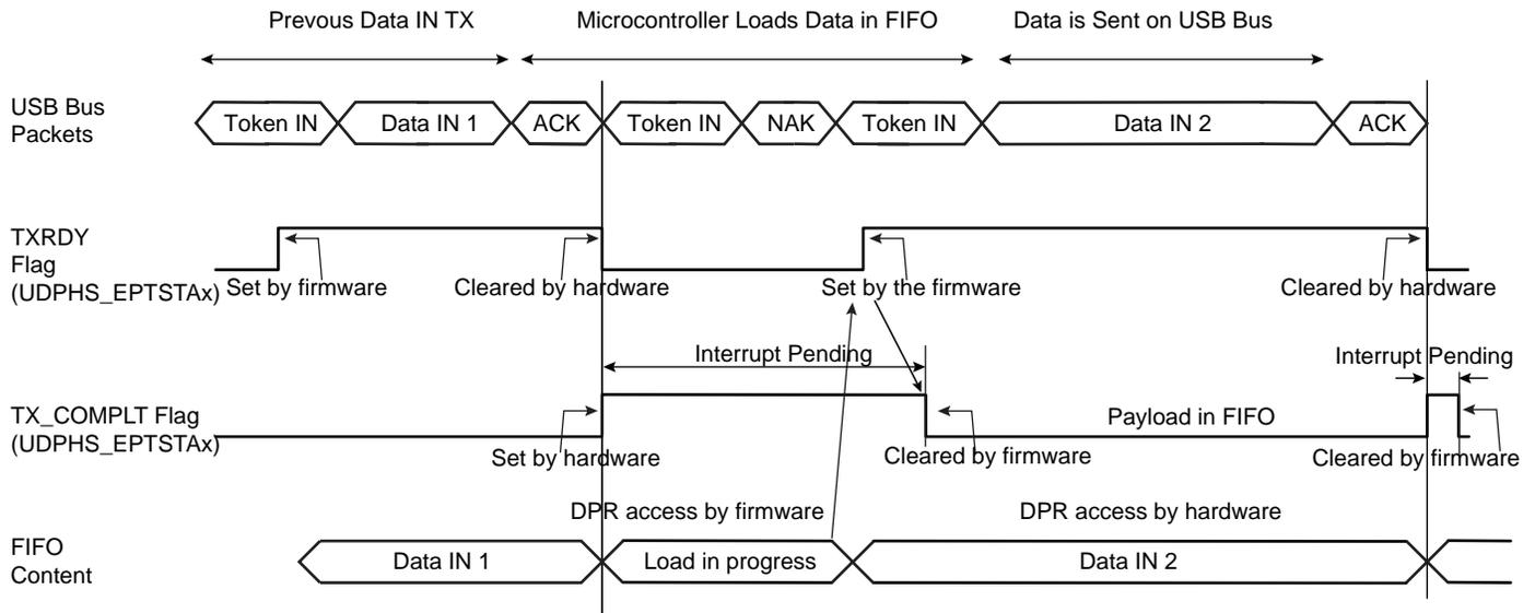
**Figure 35-10: Data IN Transfer for Endpoint with Two Banks**
