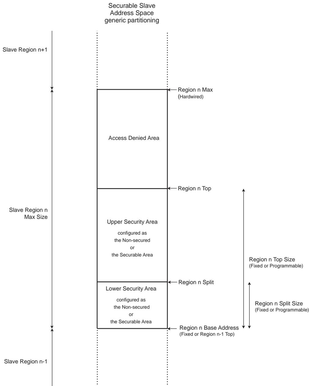
A set of Bus Matrix security registers allows to specify, for each AHB slave, slave security region or slave security area, the security mode required for accessing this slave, slave security region or slave security area.
