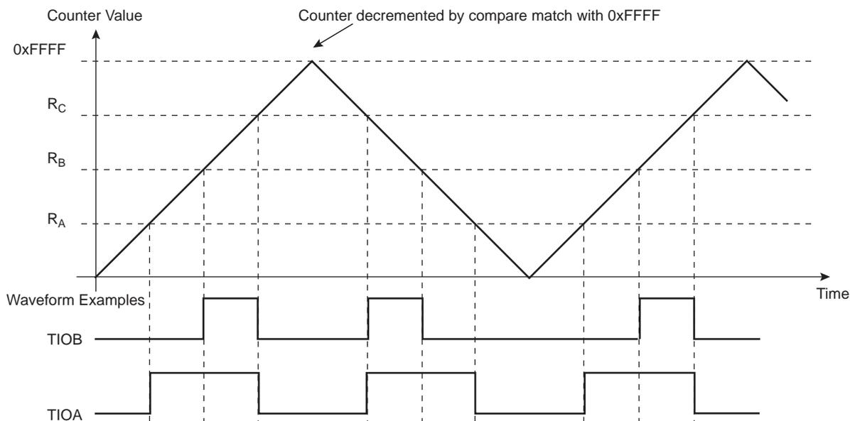
**Figure 46-12: WAVSEL = 01 with Trigger**
