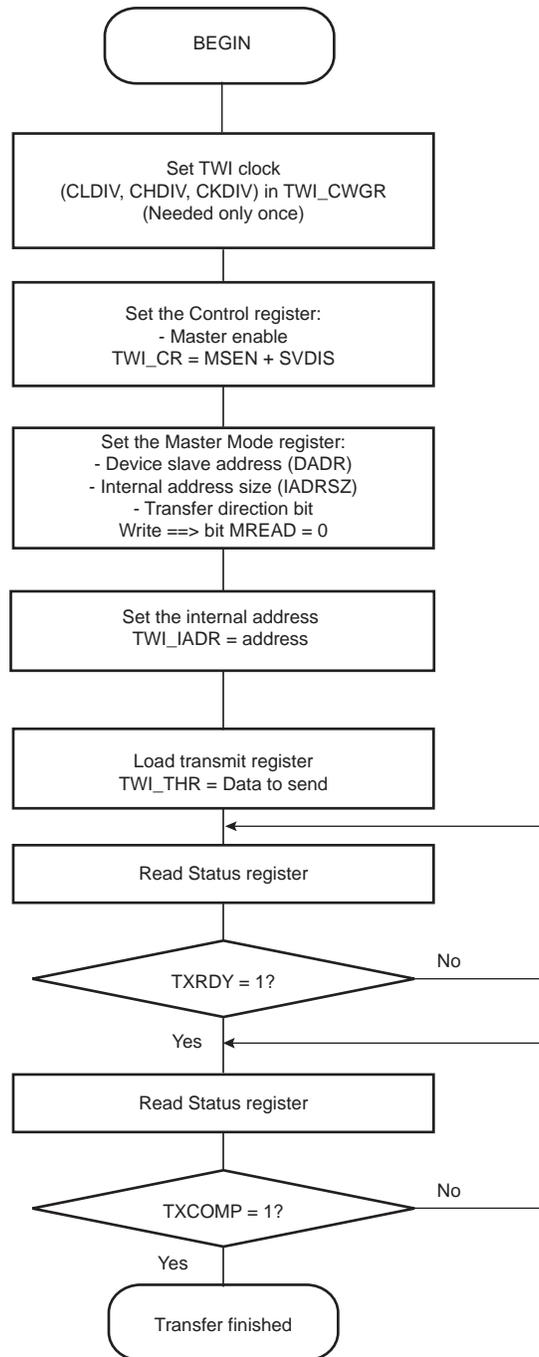
**Figure 40-15: TWI Write Operation with Multiple Data Bytes with or without Internal Address**
