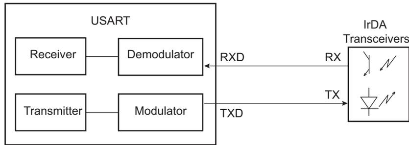
The receiver and the transmitter must be enabled or disabled depending on the direction of the transmission to be managed.
