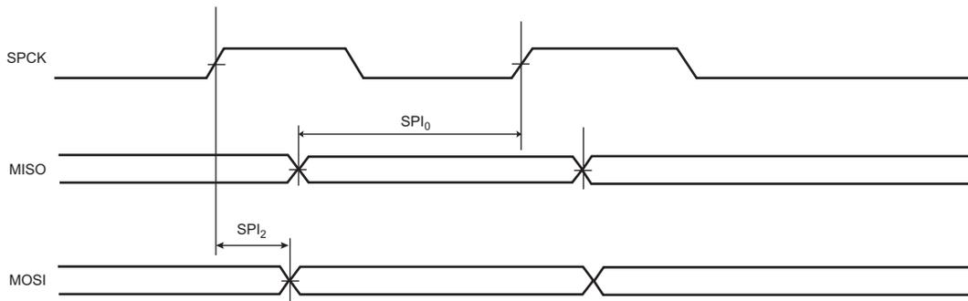
**Figure 56-7: SPI Master Mode 0 and 3**
