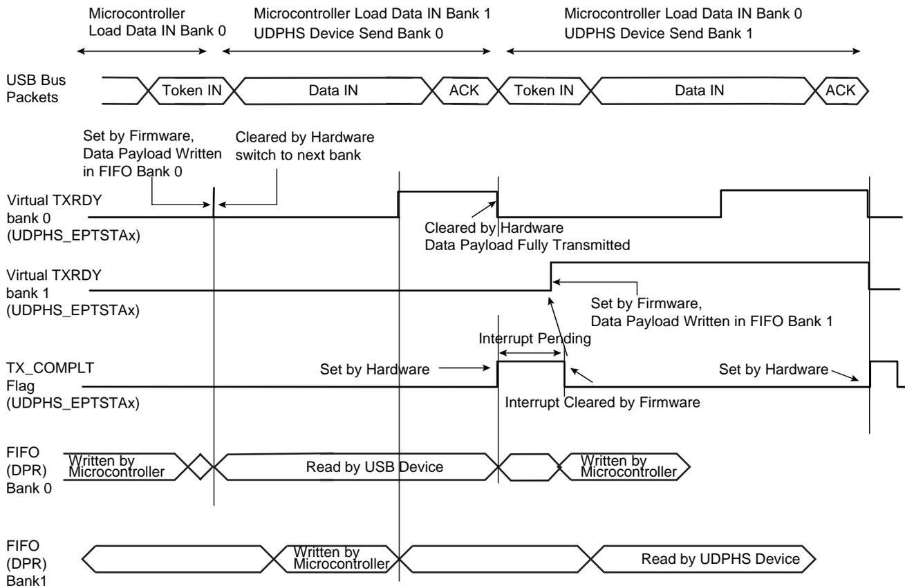
**Figure 35-11: Data IN Followed By Status OUT Transfer at the End of a Control Transfer**
