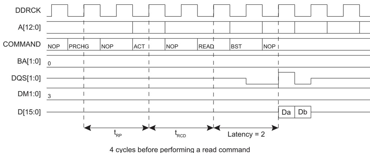
The multiport controller is designed to mask these timings and thus improve the bandwidth of the system.
