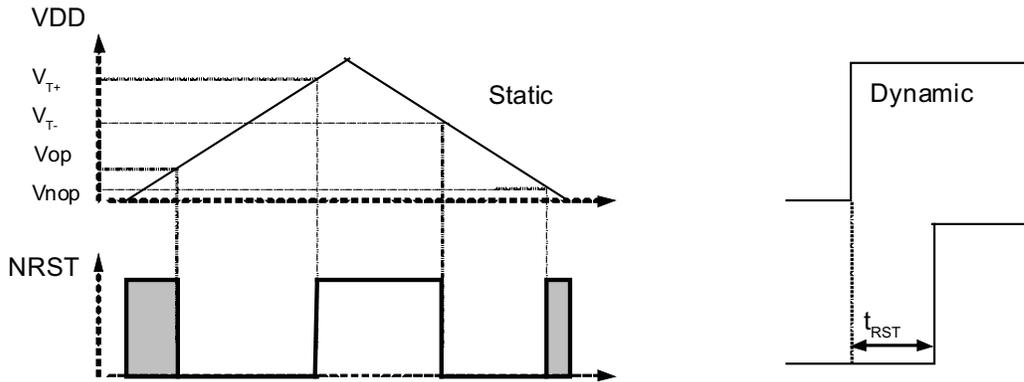
When a very slow (versus  $t_{RST}$ ) supply rising slope is applied on POR VDD pin, the reset time becomes negligible and the reset signal is released when VDD rises higher than  $V_{T+}$ .
