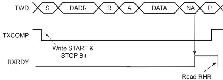
**Figure 40-8: Master Read with Multiple Data Bytes**
