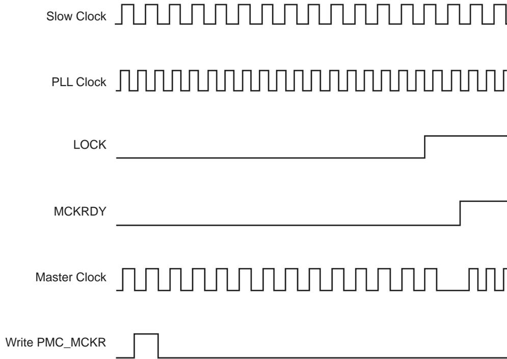
**Figure 27-8: Switch Master Clock from Main Clock to Slow Clock**
