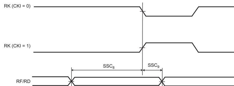
**Figure 56-18: SSC Receiver, RK in Input and RF in Output**
