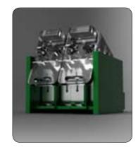
Insulation **Displacement** Intended for use in industrial communications and control applications such as analog or serial communications using 22-24 awg wire. Pivot block plug mates with 3.5mm horizontal and vertical terminal block headers.
