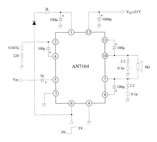
Note) Please take note if the external circuit used is by following the test circuit, the standby function may misoperate and IC cannot function.
