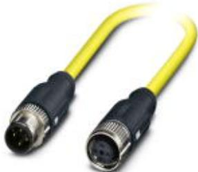
Sensor/Actuator cable, 4-position, PVC, Yellow RAL 1021, shielded, Plug straight M12-SPEEDCON, A-coded, on Socket straight M12-SPEEDCON, A-coded, Cable length: 1.5 m
