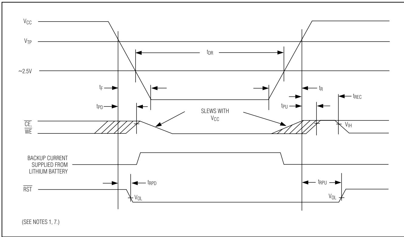
**Note 1:** RST is an open-drain output and cannot source current. An external pullup resistor should be connected to this pin to realize a logic-high level.
