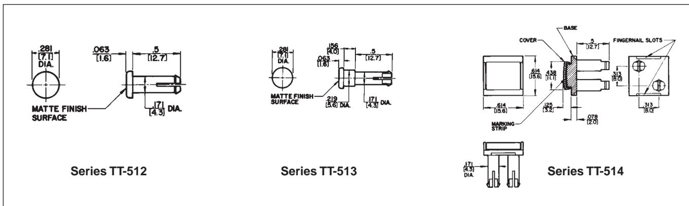
DIMENSIONS ARE FOR REFERENCE ONLY  $\frac{\text{Inch}}{\text{(mm)}}$
