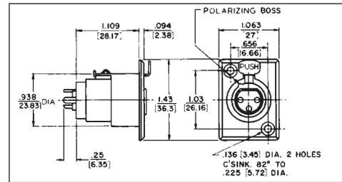
Studio quality black and gold Q-G® receptacle with black housing and gold contacts is designed for low/stable contact resistance and withstands corrosion where highest quality is required for recording and broadcast studio equipment, consoles, and other applications.
