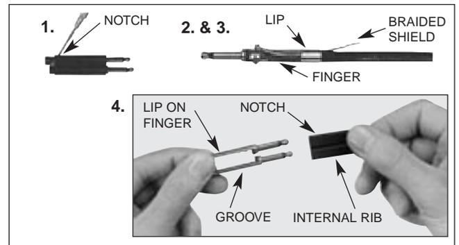
**4. ASSEMBLY:** Align grooves in fingers with internal handle ribs and insert fingers into rear of handle. Push fingers in until lips or rear of fingers snap into notches on handle.
