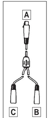
Series 391Q Y-Adapters can combine or split typical audio signals using a combination of Switchcraft Q-G® A3F and A3M cord plugs. Outputs of two microphones can conveniently be connected in parallel and connected to a single input using a 391Q23 Y-Adapter. Cabling is 2-conductor shielded, 2-foot long gray jacket with molded Y-junction at center point. Mates with Switchcraft Q-G® and QGP® connectors.
