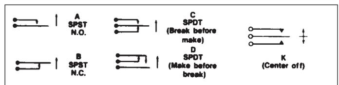
The above are strictly electrical schematics and do not necessarily indicate relative solder lug positions.
