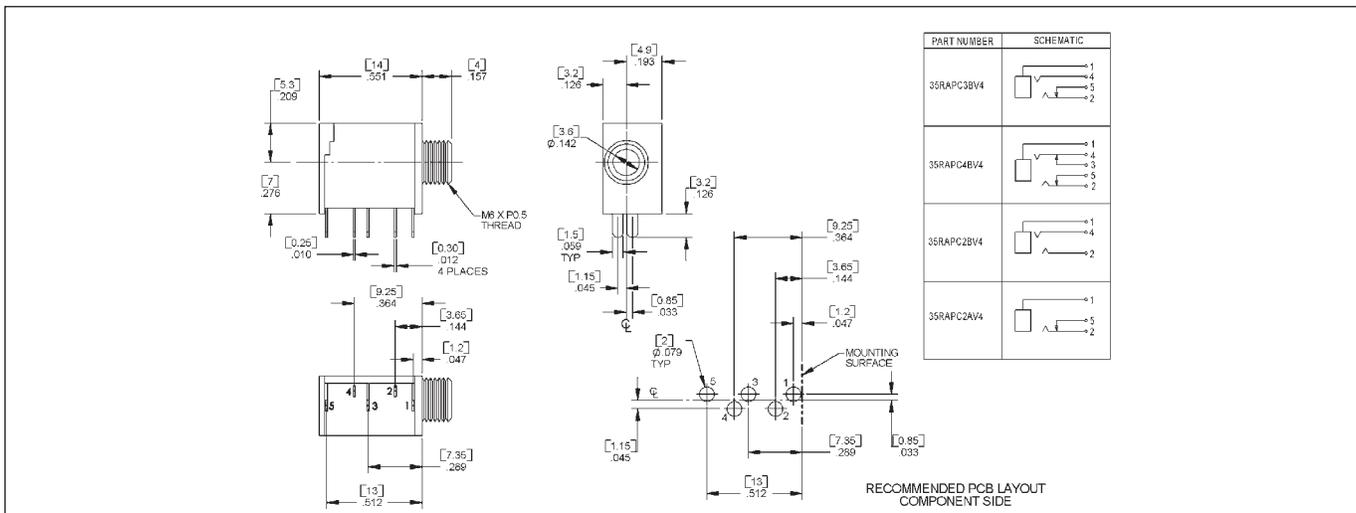
DIMENSIONS ARE FOR REFERENCE ONLY  $\frac{\text{Inch}}{\text{(mm)}}$
