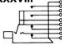
Double closed circuit. Isolated switching—Two "make" circuits.
