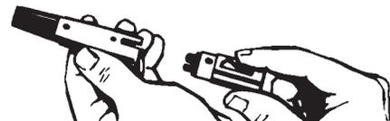
Insert assembly is now readily removed from shell. Note "Ground Terminal" area – large soldering cups make cable installation fast and easy. Unitized 1-piece insert eliminates possible loss of latchlock and spring.
