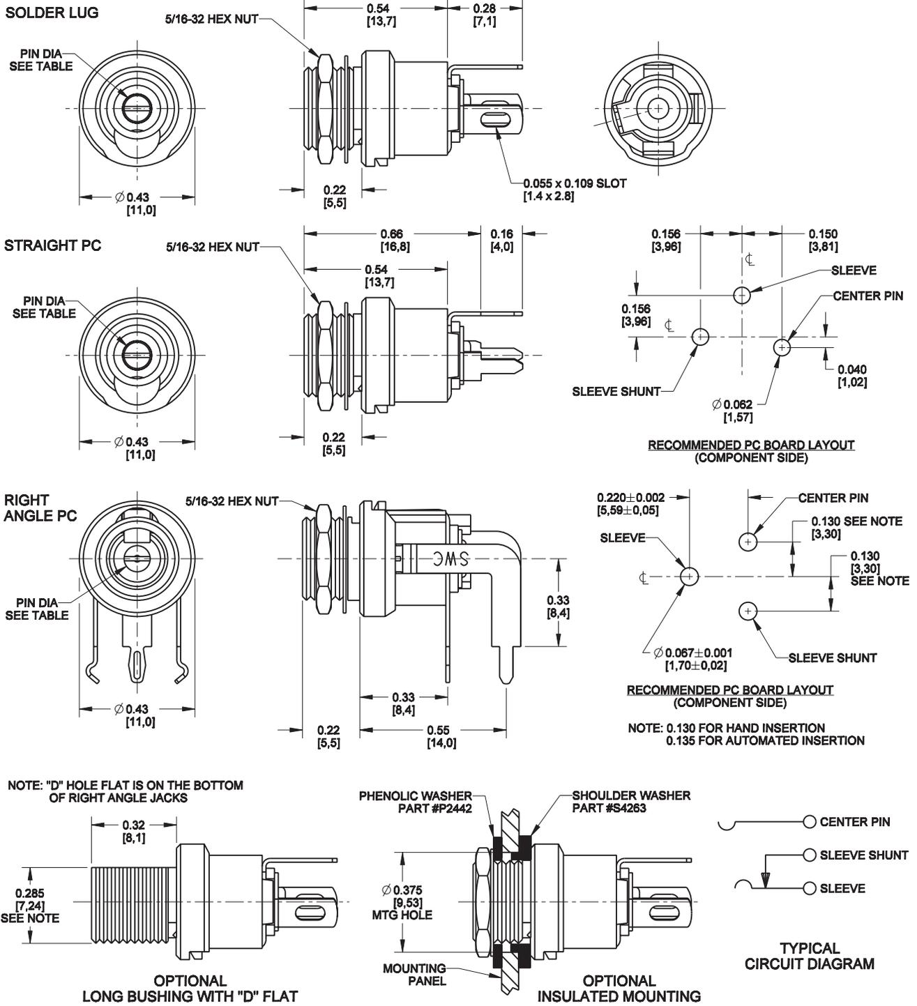
DIMENSIONS ARE FOR REFERENCE ONLY  $\frac{\text{Inch}}{(\text{mm})}$
