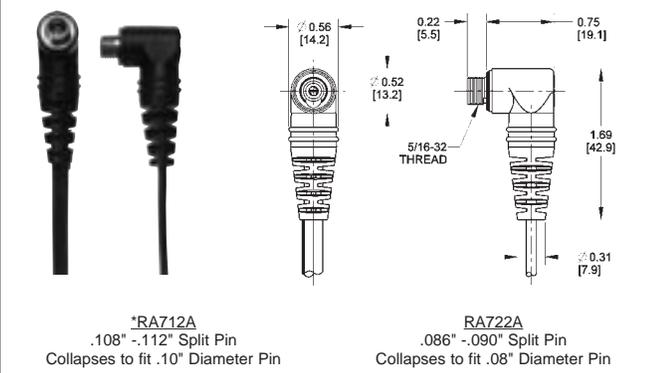
DIMENSIONS ARE FOR REFERENCE ONLY  $\frac{\text{Inch}}{(\text{mm})}$
