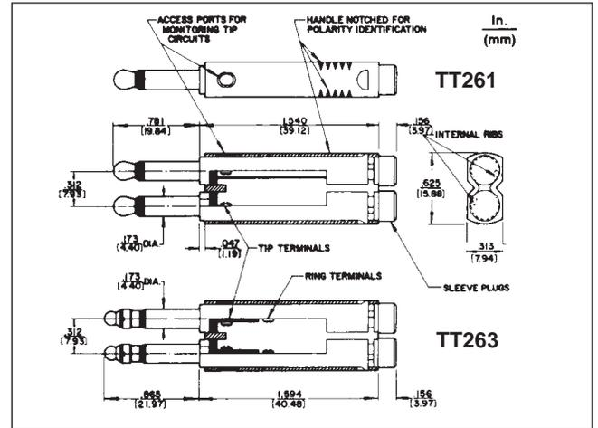
**TT263:** 6-circuit plug consists of two electrically-independent 3-conductor fingers with black handle. Can use single or dual cables for two electrically-independent 3-conductor fingers or common tip, ring and/or sleeve circuits.
