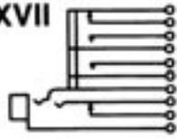
Tip closed; ring open circuits. Isolated switching—two "make" circuits and one "break" circuit. (J10-2A-1B).
