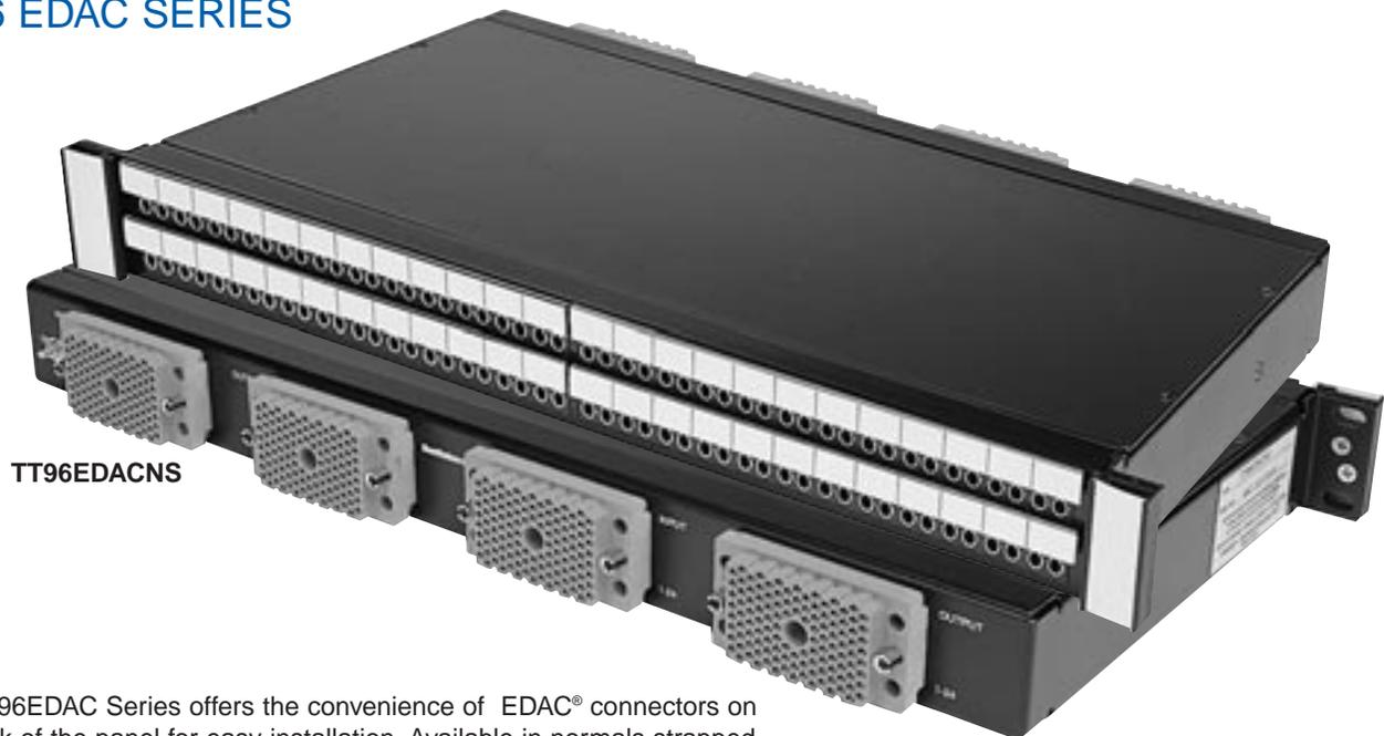
The TT96EDAC Series offers the convenience of EDAC® connectors on the back of the panel for easy installation. Available in normals strapped and normals brought out, both wired to the SAC code of wiring. We also offer custom wiring configurations. Contact the factory for details.
