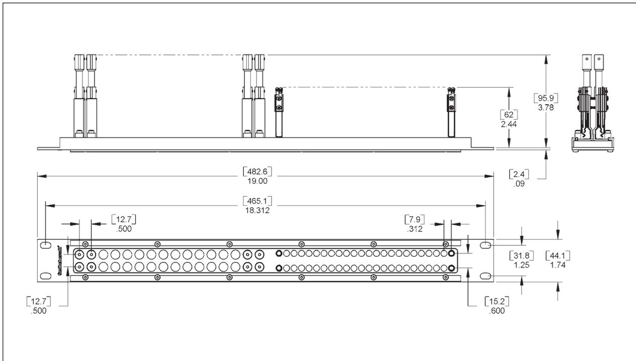
DIMENSIONS ARE FOR REFERENCE ONLY  $\frac{\text{Inch}}{(\text{mm})}$
