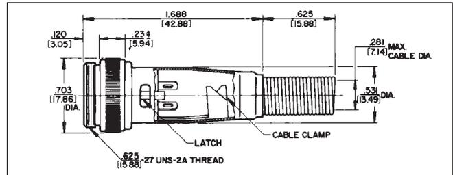
Non-reflective metal shell; coupling ring; 2 through 5 pins (male) or 2 through 5 contacts (female). Also 2-, 3- and 4-contact inserts with two shunted (N.C.) contacts. Efficient cable clamp and strain relief.
