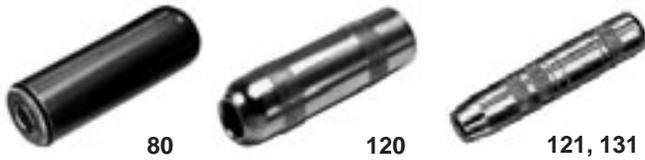
Extension Jax® jacks are connected to the end of a cable. 2- and 3-conductor jacks mate with standard commercial phone plugs, and have a sturdy cable clamp strain relief, knurled shielded or molded black plastic handles, and a screw type solder terminal. All internal parts are interlocked. Note: See locking phone plugs section.
