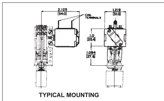
DIMENSIONS ARE FOR REFERENCE ONLY  $\frac{\text{Inch}}{\text{(mm)}}$
