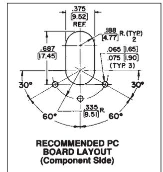
DIMENSIONS ARE FOR REFERENCE ONLY  $\frac{\text{Inch}}{\text{(mm)}}$
