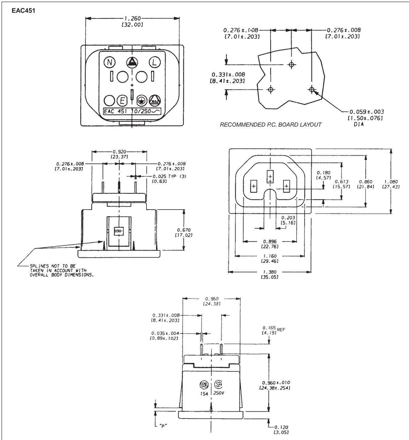
DIMENSIONS ARE FOR REFERENCE ONLY  $\frac{\text{Inch}}{\text{(mm)}}$
