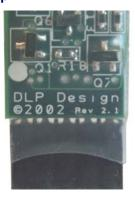
Even though Ubicom-based hardware designs only require four pins to properly interface to the DLP-FLASH programmer, it is recommended that all designs use a 5-pin header in order to help prevent possible improper connection to the programmer.
