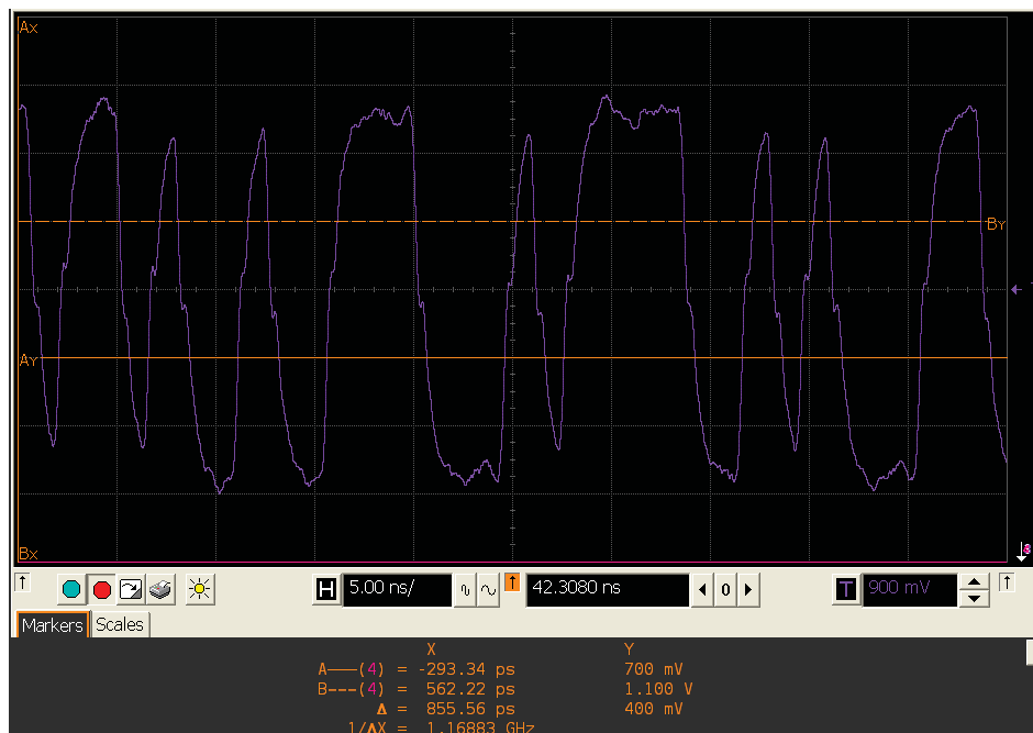
Figure 7-33: DDR2 DIMM Read HW Measurement - Waveform Scope Shot at Probe Point (FPGA1 Via)
